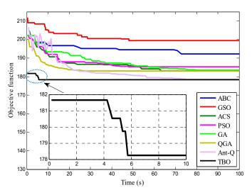
**Figure 9.** Convergence of the fourth new task of the IEEE 300-bus system obtained in the online optimization.
