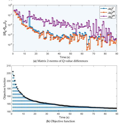
**Figure 7.** Convergence of the eighth source task of the IEEE 300-bus system obtained in the pre-learning process.
