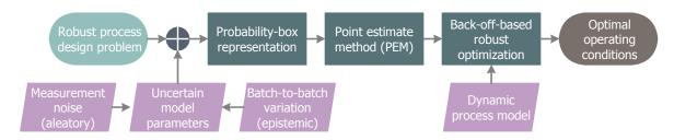
Figure 1. Flowchart of the proposed framework of robust process design under batch-to-batch variation.
