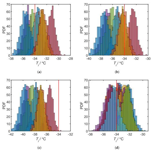
**Figure 5.** Probability density functions of the temperature at the sublimation interface ( $T_i$ ) obtained from different probability distributions of parameter uncertainties for (**a**) nominal, (**b**) robust, (**c**) p-box robust (plausibility function), and (**d**) p-box robust (belief function) process designs. The red line is the upper limit of  $T_i$ .
