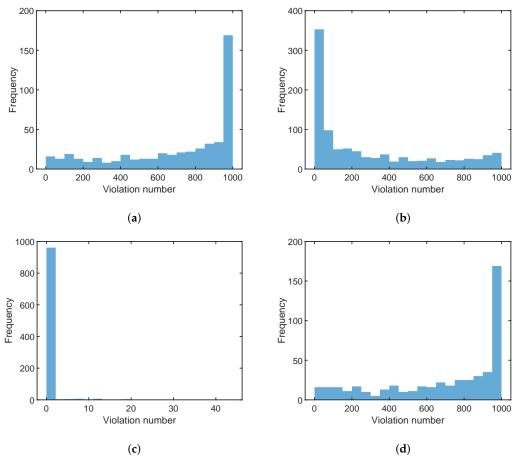
**Figure 6.** Normalized histograms of constraint violations for the (**a**) nominal, (**b**) robust, (**c**) p-box robust (plausibility function), and (**d**) p-box robust (belief function) process designs.
