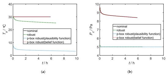
**Figure 4.** Designed profiles for the shelf temperature  $T_s$  (**a**) and the chamber pressure  $P_c$  (**b**) of the nominal, robust, p-box (plausibility function) robust, and p-box (belief function) robust designs.
