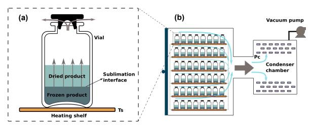
**Figure 3.** Illustration of the freeze-drying process. Model parameters can represent the dynamic processes of a single vial (**a**) appropriately, but may fail for all vials that are handled in the freeze-dryer (**b**) due to batch-to-batch variations.
