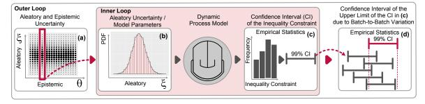
**Figure 2.** Illustration of the outer and inner loop setting for evaluating the inequality constraint under aleatory and epistemic uncertainty. Sampling from epistemic uncertainty (**a**) results in aleatory uncertainty realization (**b**), which is propagated to the inequality constraint (**c**) via the process model. Re-sampling from the epistemic uncertainty (**a**) helps to quantify the variation in the upper limit of the inequality constraint (**d**).
