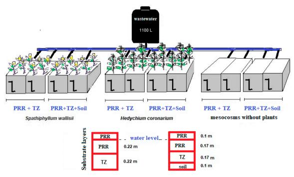
Figure 1. Schematic of the mesocosms wetland study.
