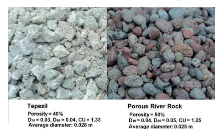
Figure 2. Materials used as filter media in the constructed wetlands (CWs) in this study.
