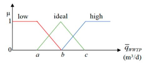
**Figure 7.** Fuzzy sets for  $\overline{q}_{WWTP}$ .
