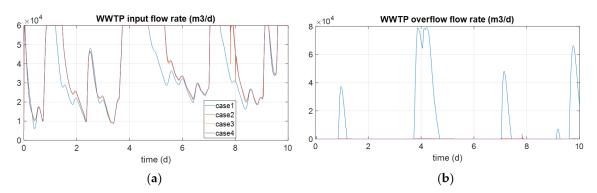
Figure 15. WWTP input (a) and overflow flow rates (b).
