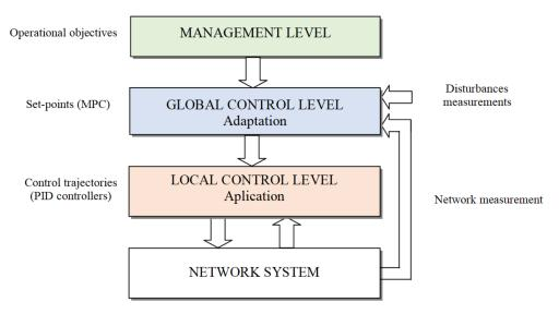
Figure 5. Hierarchical control system.
