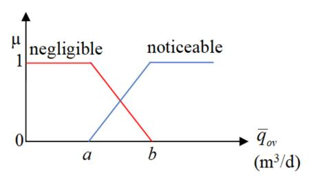
**Figure 8.** Fuzzy sets for  $\overline{q}_{ov}$ .
