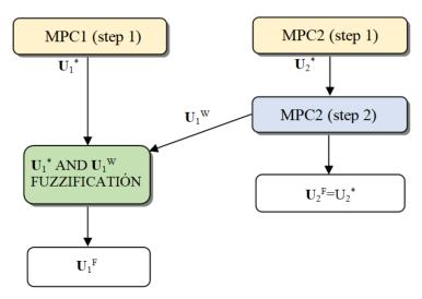
Figure 6. Distributed Model Predictive Control (DMPC) algorithm.
