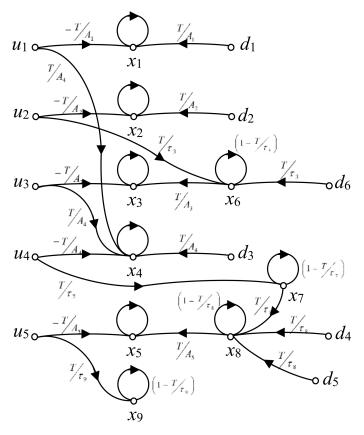
Figure 3. Direct graph of the sewer.
