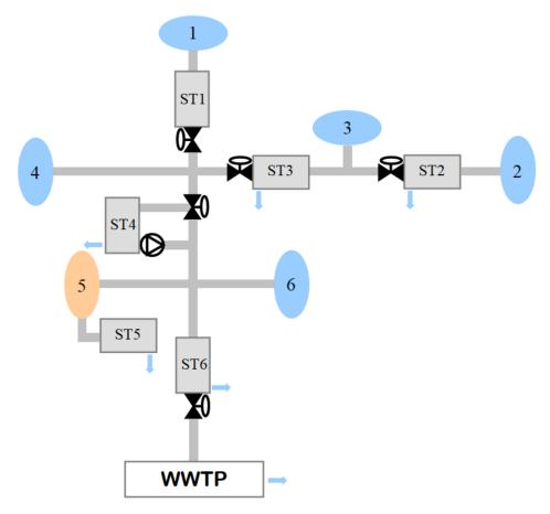
Figure 1. Catchment and sewer system.
