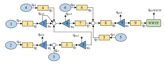
Figure 2. Simplified sewer block diagram.
