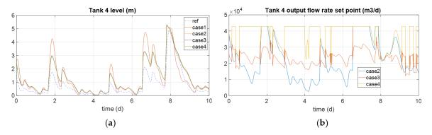
Figure 13. Tank 4 level (a) and output flow rate set point (b).
