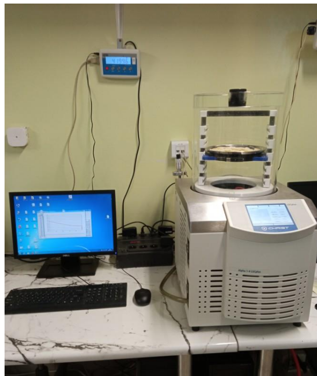
Figure 2. Measuring stand for the recording of mass changes of sample during FD.
