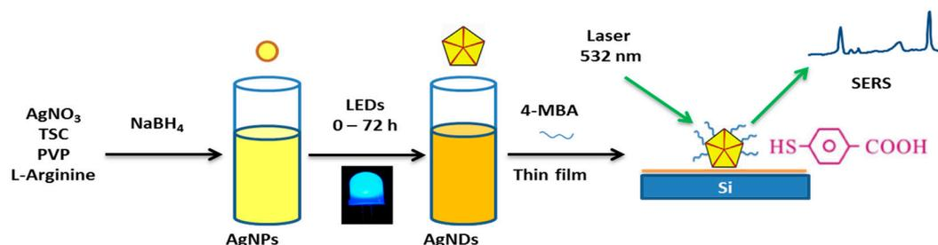
**Figure 1.** Schematic illustration of the fabrication and surface-enhanced Raman scattering (SERS) measurement of nanodecahedrons (AgNDs). TSC: trisodium citrate tribasic dihydrate, PVP: polyvinylpyrrolidone, AgNPs: silver nanoplates, LEDs: light-emitting diodes, 4-MBA: 4-mercapto benzoic acid.
