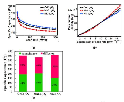
**Figure 5.** (a) Specific capacitance vs. scan rate, (b) and peak current vs. (scan rate) $^{1/2}$ , and (c) diffusion and capacitive contribution to the specific capacitance.
