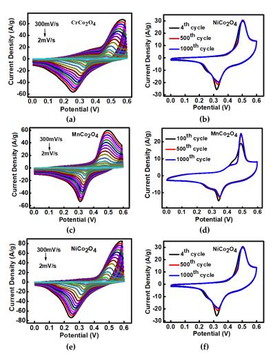
**Figure 4.** (**a**,**c**,**e**) show cyclic voltammetry curves of tubular  $MCo_2O_4$  (M = Cr, Mn, Ni) electrode obtained in the scan range of 5 mV/s to 300 mV/s measured in 3M KOH electrolyte. (**b**,**d**,**f**) show cyclic stability curves measured up to 1000 cycles in 3M KOH electrolyte at scan rate of 40 mV/s.
