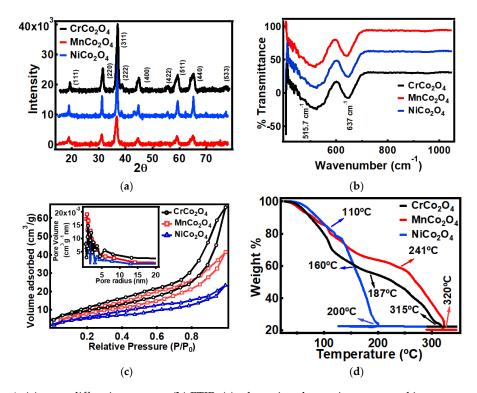
**Figure 1.** (a) x-ray diffraction pattern, (b) FTIR, (c) adsorption-desorption curve and inset pore volume distribution, and (d) thermogravimetric curve of tubular  $MCo_2O_4$  (M = Cr, Mn, Ni) structures.
