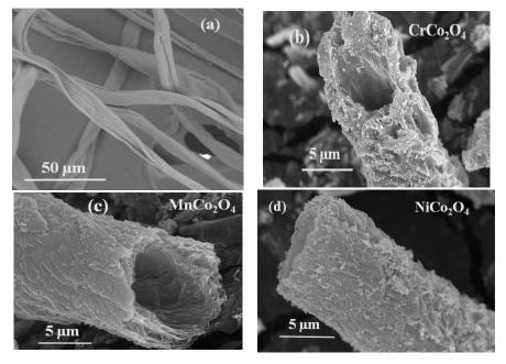
**Figure 2.** SEM images of (a) cotton fiber, (b), (c), and (d) bio-templated tubular  $MCo_2O_4$  (M = Cr, Mn, Ni) structures.
