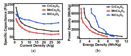
**Figure 7.** (a) Comparison of specific capacitance as a function of current density and (b) Ragone plot of power density vs. energy density.
