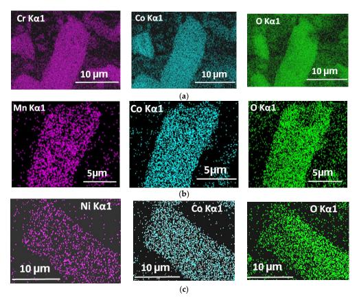
**Figure 3.** (a), (b), and (c) shows EDX mapping of tubular MCo<sub>2</sub>O<sub>4</sub> (M = Cr, Mn, Ni) structures, respectively.
