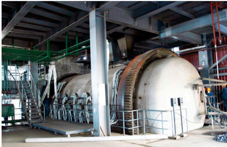
Figure 9. Commercial SKS smelting furnace in the Fangyuan 1<sup>#</sup> phase smelter.
