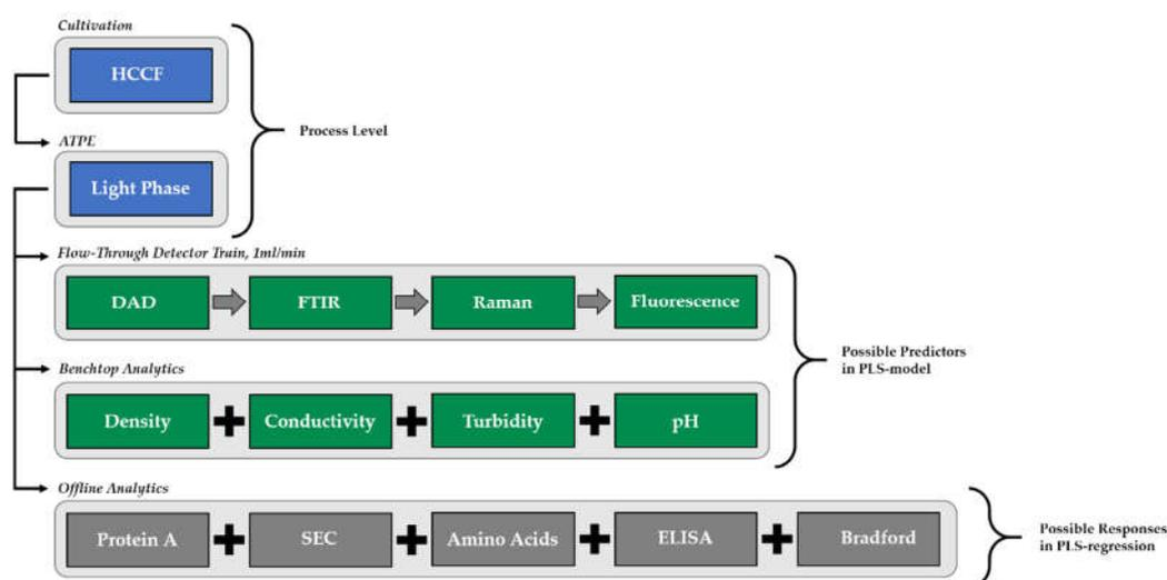
**Figure 4.** Experimental set-up (blue) and analytical procedure (green). Harvested cell culture fluid (HCCF) is from start ( $t_0$ ) to end of cultivation ( $t_{10}$ ) processed by aqueous two-phase extraction (ATPE). The antibody containing light phase is pumped in the detector array for spectral analysis and investigated in PLSR as predictors. Offline analytics (grey) are investigated as responses.
