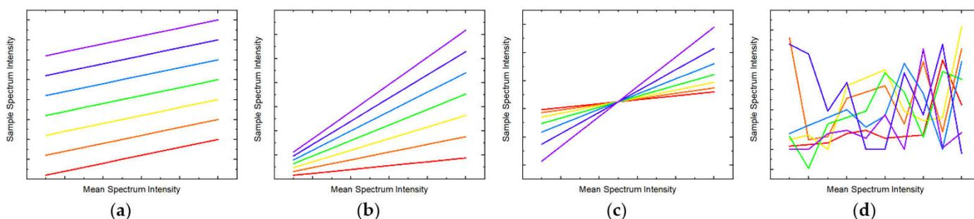
**Figure 5.** Exemplary scatter effects plots of (a) additive effects, (b) scatter effects, (c) additive and scatter effects, and (d) complex effects. Colors indicate spectra from different samples.
