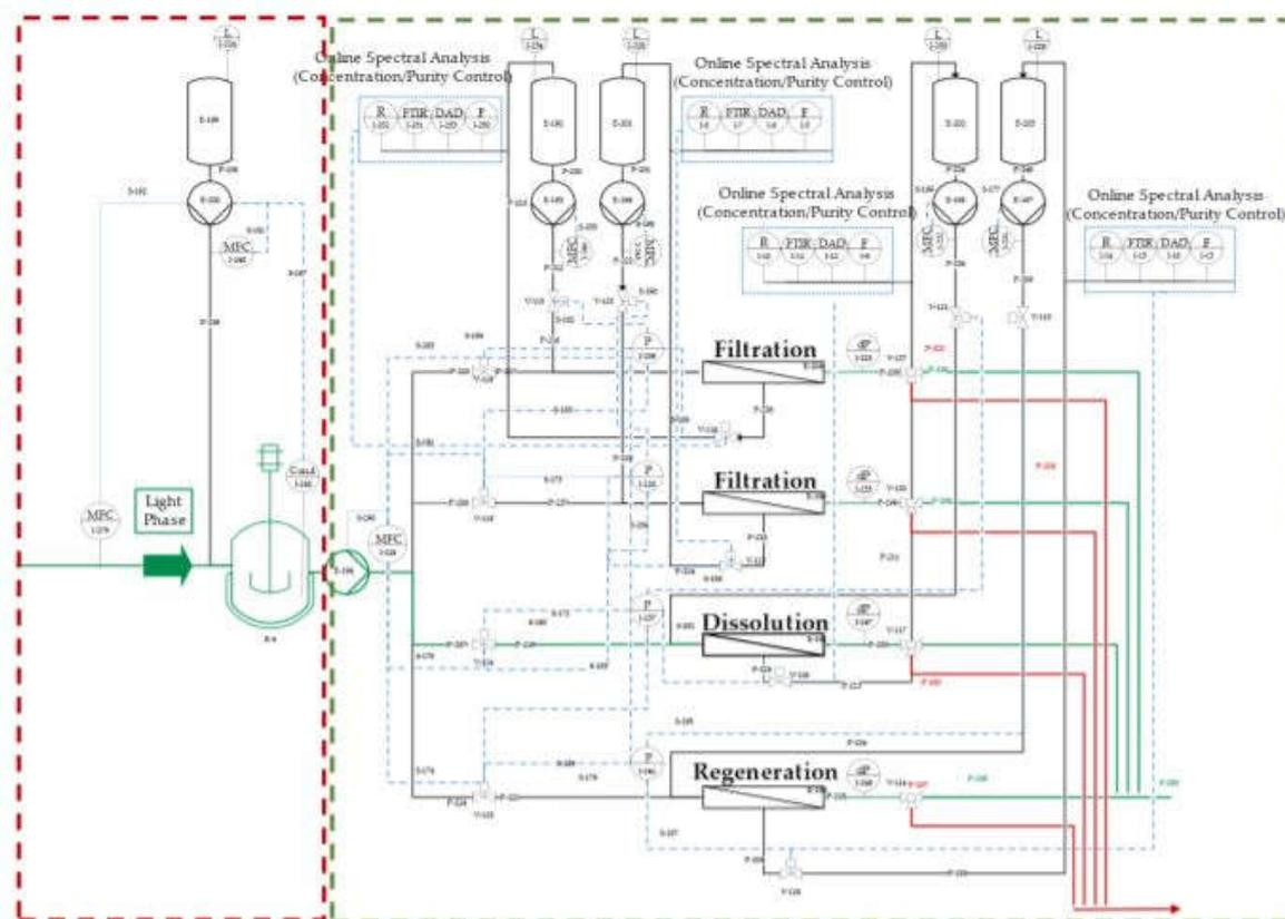
**Figure 19.** Process control strategy for precipitation. A PAT measurement array at the outlet of the ATPE forwards mAb and side component concentrations to the precipitation unit, which adjusts filtration and dissolution times to obtain a constant mAb concentration in the dissolution solution.
