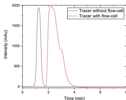
**Figure 8.** Tracer chromatogram with and without Raman flow-cell.
