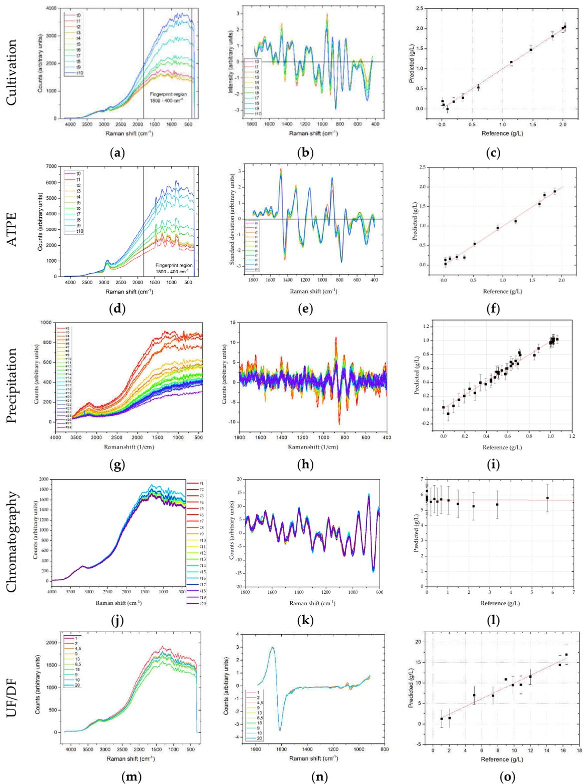
**Figure 7.** Raman spectra: raw (a,d,g,j,m), after preprocessing (b,e,h,k,n) and PLSR results (c,f,i,l,o). Spectra are color-coded from high concentration (blue) to low concentration (red).
