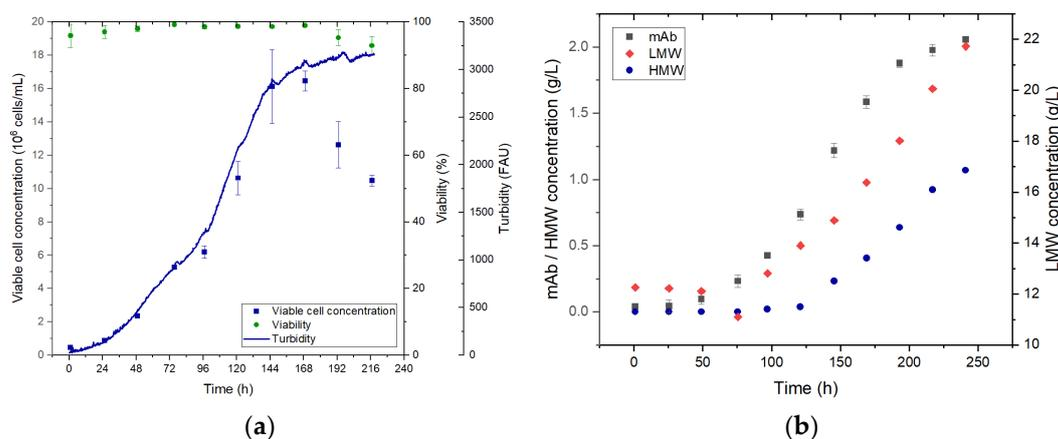
**Figure 6.** (a) Viable cell concentration, viability and turbidity over process time. (b) mAb concentration and HMW/LMW pseudo-concentrations over process time.
