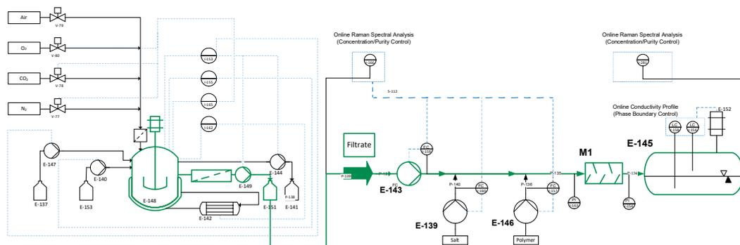
**Figure 18.** Proposed control strategy for USP and ATPE. A Raman probe is used as (PAT) at the filtrate outlet of USP and forwards mAb and side component concentrations to the ATPE, which adjusts the polymer and salt concentrations to produce light phase with a constant mAb concentration which is then forwarded to the precipitation unit.
