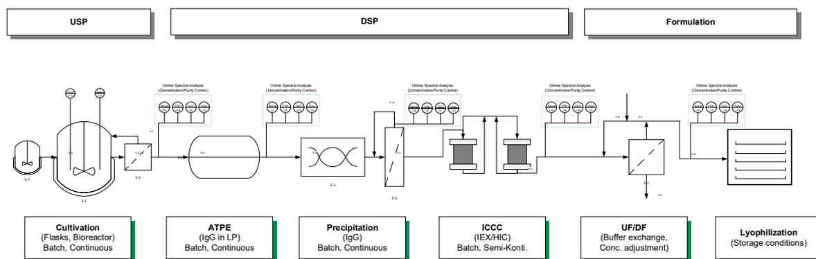
**Figure 3.** Proposed process flow sheet including spectroscopic PAT sensors. A PAT measurement array is placed at the outlet of each unit operation to provide real time data on monoclonal antibody (mAb), high molecular weight (HMW) impurities, and light molecular weight (LMW) impurity concentrations that are then used as input for the process model, which calculates the necessary process adjustments to ensure operation within a pre-defined design space.
