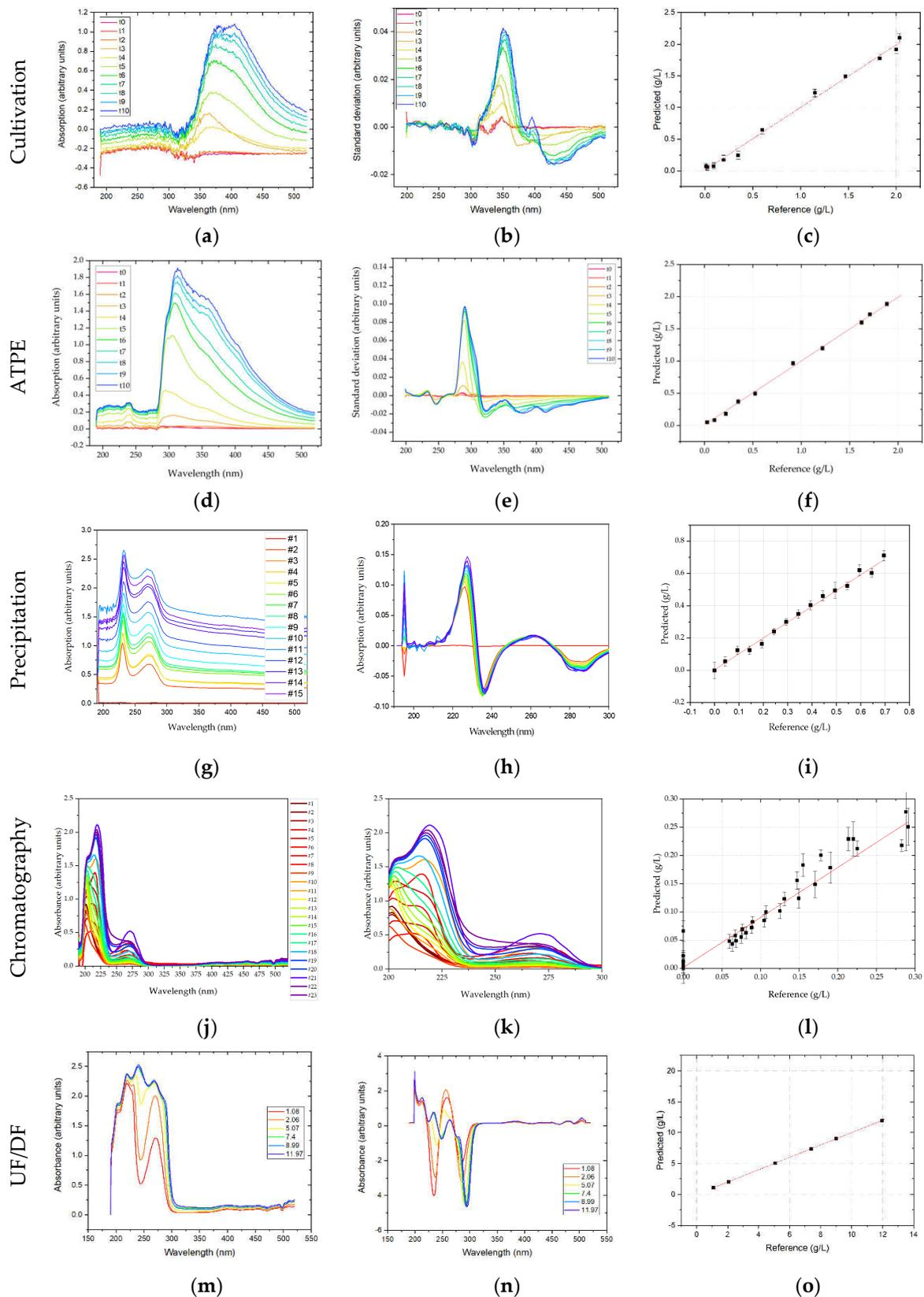
**Figure 10.** DAD spectra: raw (a,d,g,j,m), after preprocessing (b,e,h,k,n) and PLSR results (c,f,i,l,o). Spectra are color-coded from high concentration (blue) to low concentration (red).
