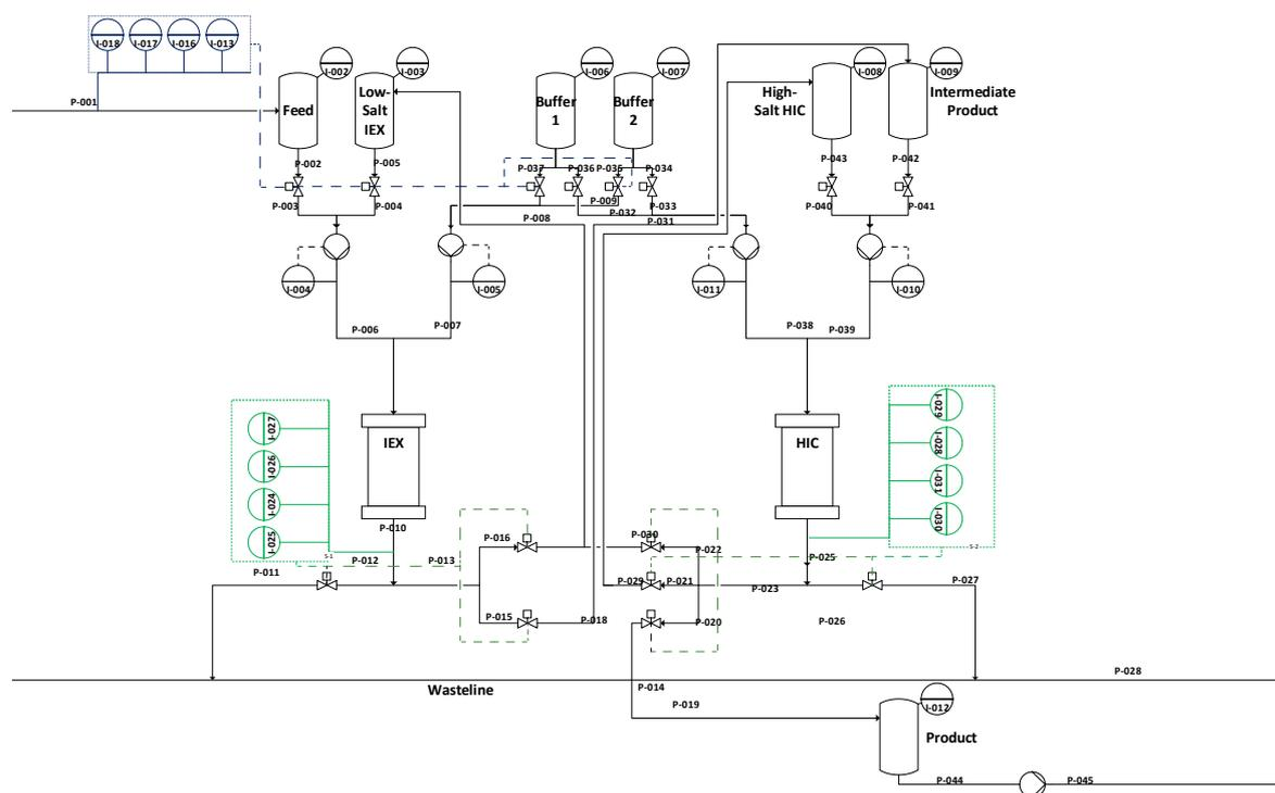
**Figure 20.** Proposed control strategy for iCCC. PAT measurement information from the precipitation outlet (top left, blue) is used to control the loading time of the IEX. Fractionation in the IEX can also be monitored and controlled by the described PAT detectors (green).
