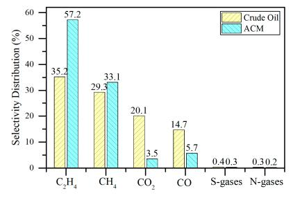
**Figure 13.** Selectivity distribution of gaseous products released from pyrolysis of crude oil in the presence and absence of activated carbon modified with 5.0 wt.% of magnetite nanoparticles (ACM).
