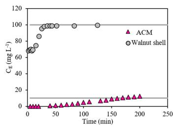
**Figure 11.** Breakthrough curves for the walnut shell (WH) and activated carbon modified with 5.0 wt.% of magnetite nanoparticles (ACM), at room temperature conditions and with an initial concentration of 100 mg  $L^{-1}$  of crude oil in water.
