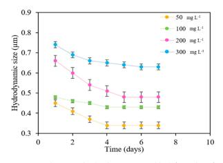
**Figure 1.** Change in hydrodynamic size (d50) for 7 days for emulsions prepared at different crude oil concentrations between 50 and 300 mg  $L^{-1}$ .
