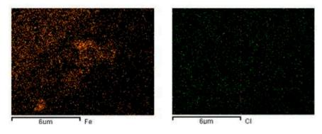
**Figure 8.** Mapping of elements present on the surface of the activated carbon modified with 5.0 wt.% of magnetite nanoparticles (ACM) sample by SEM-EDX analysis.
