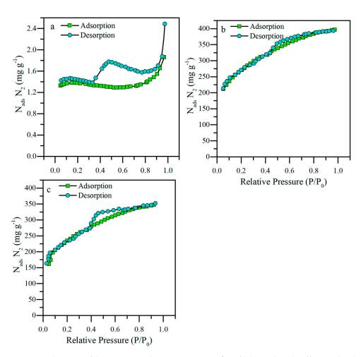
**Figure 5.** Adsorption/desorption isotherms N<sub>2</sub> at  $-196 \degree C$  of (**a**) pyrolyzed coffee residue (PCR), (**b**) synthesized activated carbon (AC) and (**c**) activated carbon modified with 5.0 wt.% of magnetite nanoparticles (ACM)
