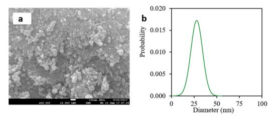
Figure 3. SEM micrograph (a) and the corresponding particle size probability distribution (b) for magnetite nanoparticles.
