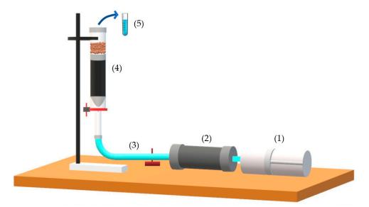
**Figure 2.** Experimental setup for dynamic adsorption tests consisting of (1) positive displacement pump, (2) cylinder, (3) regulating valves, (4) open packed-bed system and (5) effluent collection.
