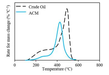
**Figure 12.** The plot of the rate for mass loss of virgin crude oil and those in the presence of activated carbon modified with magnetite nanoparticles. Crude oil adsorbed was present at 0.2 mg m<sup>-2</sup>, nitrogen flow at 100 mL min<sup>-1</sup>, a heating rate of 20 °C min<sup>-1</sup>, and the temperature uncertainty was 0.1 °C.
