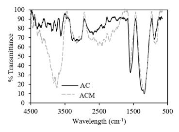
**Figure 7.** FTIR of the synthesized and modified activated carbon. The continuous line indicates the FTIR for the synthesized activated carbon (AC) material, whereas the dotted line refers to the FTIR for the activated carbon modified with 5.0 wt.% of magnetite nanoparticles (ACM) material.
