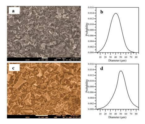
**Figure 6.** SEM micrograph of synthesized activated carbon (AC) (**a**) and activated carbon modified with 5.0 wt.% of magnetite nanoparticles (ACM) (**c**), and the corresponding particle size probability distribution of synthesized activated carbon (AC) (**b**) and activated carbon modified with 5.0 wt.% of magnetite nanoparticles (ACM) (**d**).
