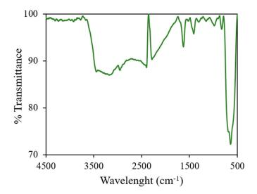
Figure 4. FTIR spectra of synthesized magnetite nanoparticles.
