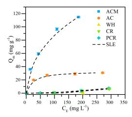
**Figure 9.** Comparison between adsorption isotherms of crude oil over walnut shell (WH), coffee residue (CR), the pyrolyzed coffee residue (PCR), the synthesized activated carbon (AC), and activated carbon modified with 5.0 wt.% of magnetite nanoparticles (ACM). pH = 7.15, temperature =  $25 \degree$ C, and the adsorbent dose was 1 g L<sup>-1</sup>.
