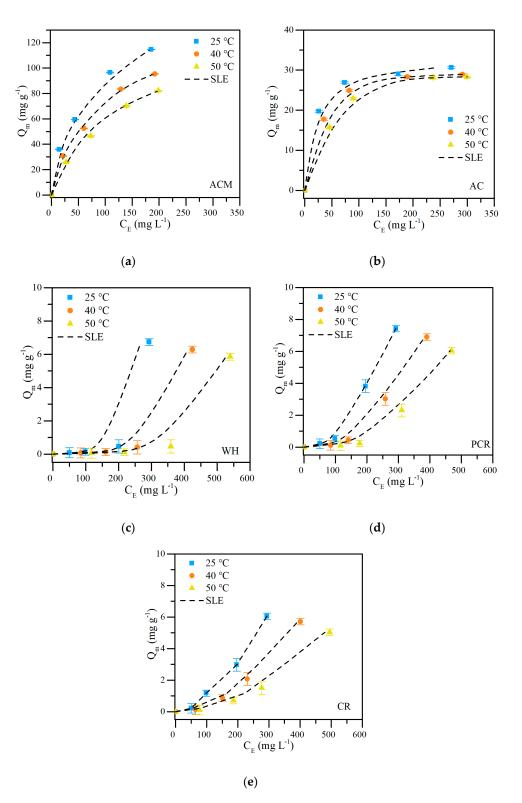
**Figure 10.** Crude oil adsorption isotherms in (**a**) activated carbon modified with 5.0 wt.% of magnetite nanoparticles (ACM), (**b**) synthesized activated carbon (AC), (**c**) walnut shell (WH), (**d**) pyrolyzed coffee residue (PCR), and (**e**) coffee residue (CR), at different temperatures of 25 °C, 40 °C and 50 °C. pH = 7.1 and the adsorbent dose was 1 g  $L^{-1}$ .
