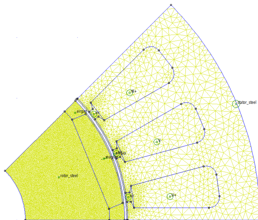
Figure 8. An example configuration for the mesh selectivity analysis. The mesh size is set to 0.18 mm on the rotor_steel, airgap, magnet regions.
