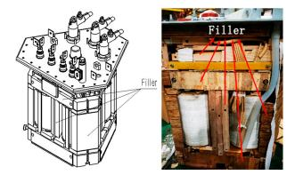
Figure 8. Filler design and actual filling effect.
