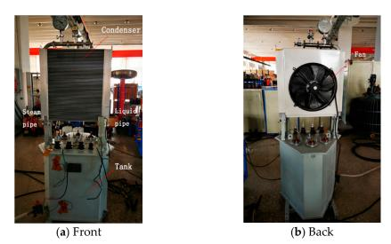
Figure 10. Prototype of evaporative cooling transformer for mine tunnels.
