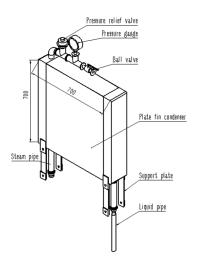
Figure 6. Assembly diagram of plate fin condenser.
