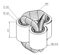
Figure 3. Core and coil structure of three-dimensional wound core transformer.
