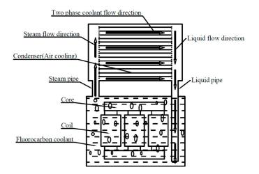
Figure 2. Schematic diagram of transformer evaporative cooling technology.
