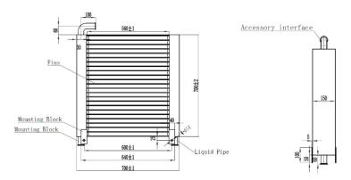
Figure 5. Condenser design drawing.
