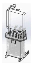
Figure 7. Design drawing of evaporative cooling transformer.
