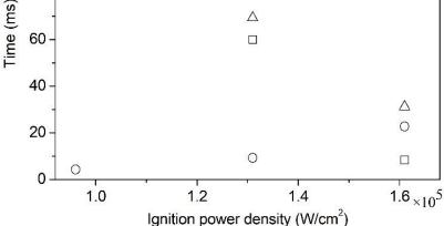
**Figure 14.** Characteristic ignition and combustion time of individual Mg microparticles at the same diameter (~65 µm) versus the laser ignition power density.
