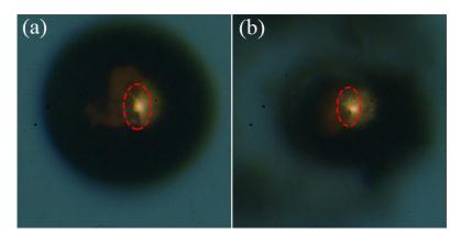
**Figure 12.** The transformation of flame structure during the combustion of individual Mg microparticle. (**a**) Flame structure before transformation, (**b**) Flame structure after transformation.
