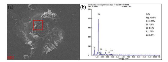
**Figure 16.** EDS spectrum of combustion residue of individual Mg microparticle, (**a**) The location of EDS analysis area in the residue (in the square box), (**b**) the content of elements, At% represents the percentage of atomic number.
