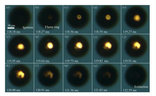
**Figure 10.** Representative snapshots of ignition and combustion stage of individual Mg microparticle. (Images acquired from Supplementary Materials, Video S1, recording frame: 11,000 fps; exposure time: 99  $\mu$ s). (a) 118.18, (b) 118.27 ms, (c) 118.36 ms, (d) 118.55 ms, (e) 119.27 ms, (f) 119.45 ms, (g) 119.64 ms, (h) 119.73 ms, (i) 119.82 ms, (j) 119.91 ms, (k) 120.00 ms, (l) 120.91 ms, (m) 121.36 ms, (n) 121.82 ms, (o) 122.55 ms.
