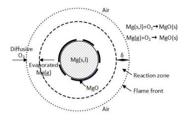
Figure 17. Schematic of physical model of individual Mg microparticle combustion.
