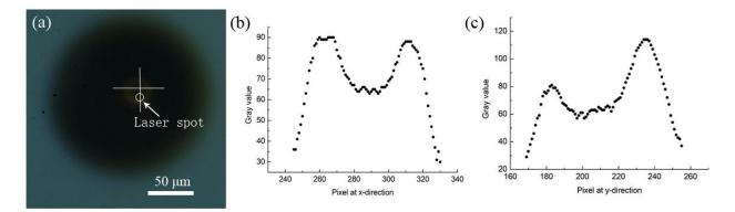
**Figure 11.** Flame structure of individual Mg microparticle, (**a**) flame picture at 118.27 ms (Figure 10 b), (**b**) gray values along central horizonal line, (**c**) gray values along central vertical line inside the flame ring structure.
