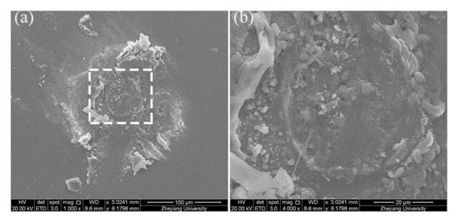
**Figure 15.** SEM photography of combustion residue of individual Mg microparticle, (**a**) the whole residue ( $1000 \times$ ), (**b**) the local residue ( $4000 \times$ ).
