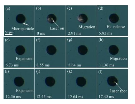
**Figure 7.** Representative snapshots of expansion and migration stage of individual Mg microparticle. (Images acquired from Supplementary Materials, Video S1, recording frame: 11,000 fps; exposure time: 99 μs). (a) Sample, (b) Laser on, 0 ms, (c) 2.91 ms, (d) 5.82 ms, (e) 6.73 ms, (f) 8.55 ms, (g) 8.64 ms, (h) 11.36 ms, (i) 12.36 ms, (j) 12.45 ms, (k) 12.64 ms, (l) 17.45 ms.
