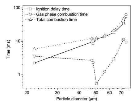
**Figure 13.** Characteristic ignition and combustion time of individual Mg microparticles at the same ignition power density  $(1.61 \times 10^5 \text{ W/cm}^2)$  against the particle diameter.
