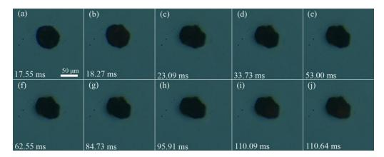
**Figure 8.** Representative snapshots of melting stage of individual Mg microparticle. (Images acquired from Supplementary Materials, Video S1, recording frame: 11,000 fps; exposure time: 99 μs). (a) 17.55, (b) 18.27 ms, (c) 23.09 ms, (d) 33.73 ms, (e) 53.00 ms, (f) 62.55 ms, (g) 84.73 ms, (h) 95.91 ms, (i) 110.09 ms, (j) 110.64 ms.
