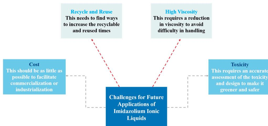
**Figure 4.** Overview of challenges for future applications in imidazolium ionic liquids.
