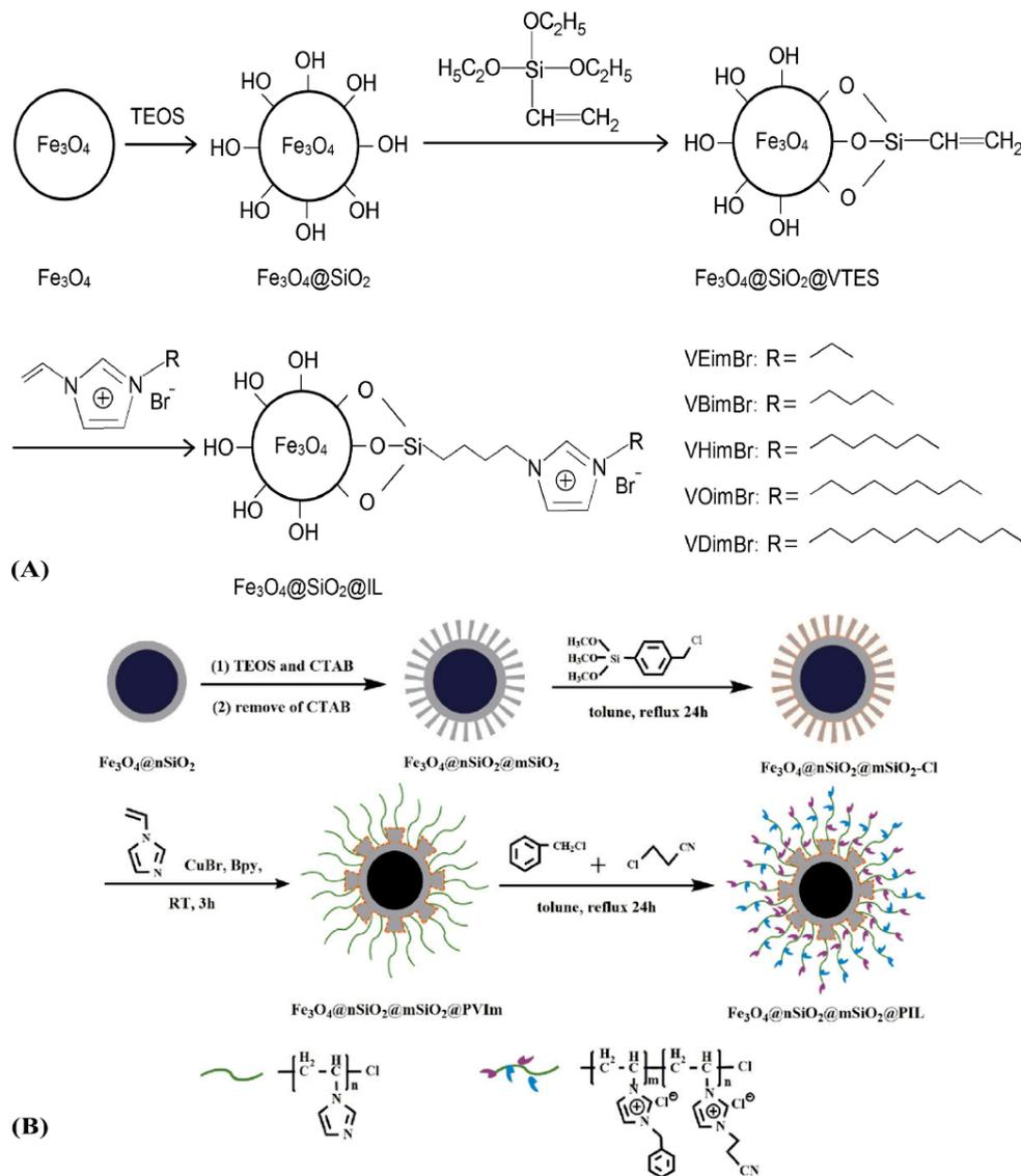
**Figure 3.** (A) Preparation procedure of  $\text{Fe}_3\text{O}_4@SiO_2@IL$  particles. Republished from Ref. [45], Copyright (2020), with permission from Elsevier. (B) Synthesis of  $\text{PILs}@mSiO_2@nSiO_2@Fe_3O_4$ . Republished from Ref. [46], Copyright (2019), with permission from Wiley.
