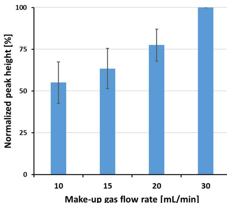
**Figure 4.** Impact of the make-up gas flow rate on the detection sensitivity of 15 compounds (10  $\mu\text{g}/\text{mL}$  each) analyzed with GC-HT-PTR-MS.
