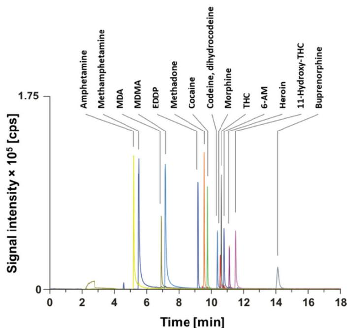
**Figure 2.** Extracted ion chromatograms obtained from the GC-HT-PTR-MS analysis of a mixture of test compounds (10 µg/mL each) employing optimized instrumental settings.
