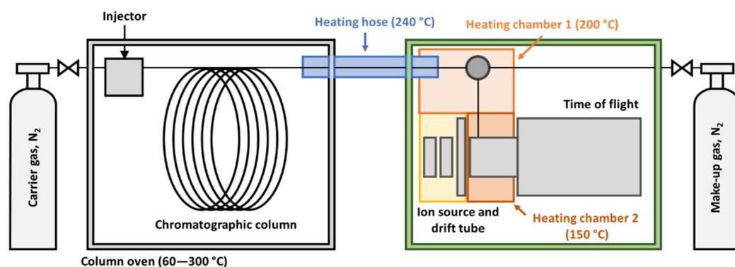
**Figure 1.** Schematic drawing of the GC-HT-PTR-MS instrument.
