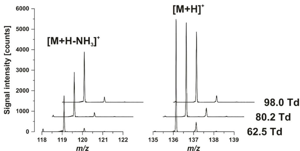
**Figure 5.** Impact of the reduced electric field strength in the drift tube on amphetamine fragmentation.
