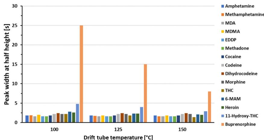
**Figure 3.** Impact of the drift tube temperature on the peak widths at half height ( $b_{0.5}$ ) of 15 compounds (10 µg/mL each) analyzed with GC-HT-PTR-MS.
