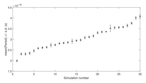
**Figure 4.** Mean and standard deviation of the Monte Carlo analysis for 30 feasible sized solutions of the DE algorithm. The best solution is the one with the lowest period (corresponding to a greater oscillation frequency).
