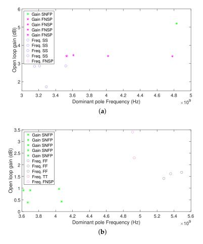
**Figure 7.** (a) Higher and (b) lower gains and dominant pole frequencies, for the solution 4 CMOS delay cell designed with UMC technology of 180 nm by applying DE algorithm.
