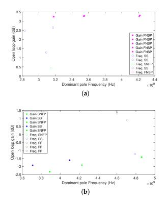
**Figure 6.** (a) Higher and (b) lower gains and dominant pole frequencies, for the solution 1 CMOS delay cell designed with United Microelectronics Corporation (UMC) technology of 180 nm by applying DE algorithm.
