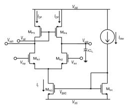
Figure 1. CMOS differential stage with active load and control voltage V<sub>ctrl</sub>.
