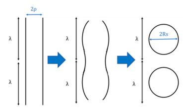
**Figure 2.** Schematic representation of a void shape evolution from a cylinder of radius  $\rho$  to two void spheres of spherical radius  $R_S$ .
