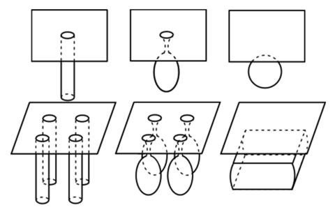
Figure 1. Scheme of the SON process without coalescence (top) and with coalescence (bottom).
