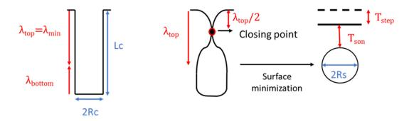
**Figure 6.** Scheme of the front and top view of the transformation from a cylindrical trench to a spherical void after annealing for  $2\pi R_C < L_C < 4\pi R_C$ .
