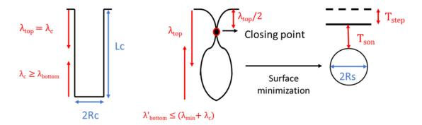
**Figure 8.** Scheme of the front and top view of the transformation from a cylindrical trench to a spherical void after annealing for  $(2^{1/2} + 1)2\pi R_C < L_C < (3 \cdot 2^{1/2} + 2)\pi R_C$ .
