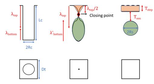
**Figure 5.** Scheme of the front and top view of the transformation from a cylindrical trench to a spherical void after annealing. Similar colored areas have the same volume.
