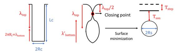
**Figure 7.** Scheme of the front and top view of the transformation from a cylindrical trench to a scheme  $4\pi R_C < L_C < (2^{1/2} + 1)2\pi R_C$ .
