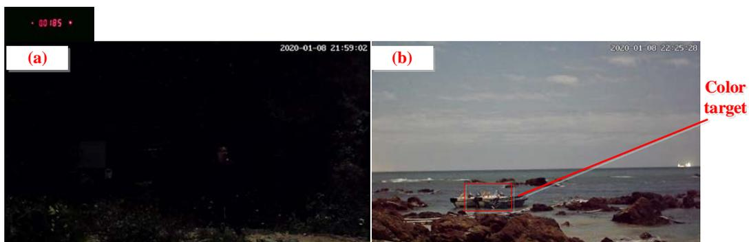
Figure 16. (a) Image captured by conventional camera; (b) image captured by the low-light imaging system.
