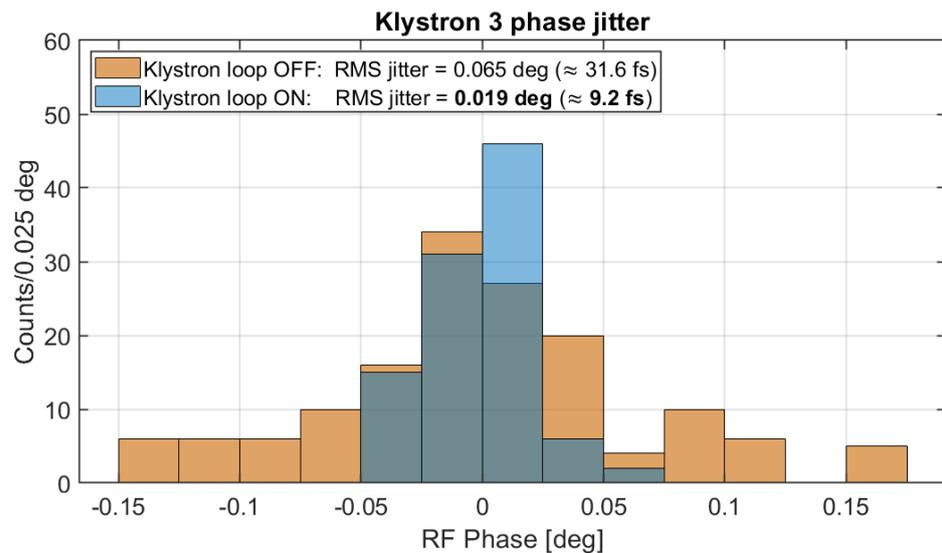
**Figure 6.** Intra-pulse feedback prototype measurement results at SPARC\_LAB facility on the C-band power plant. In bold the results obtained with the new feedback on.
