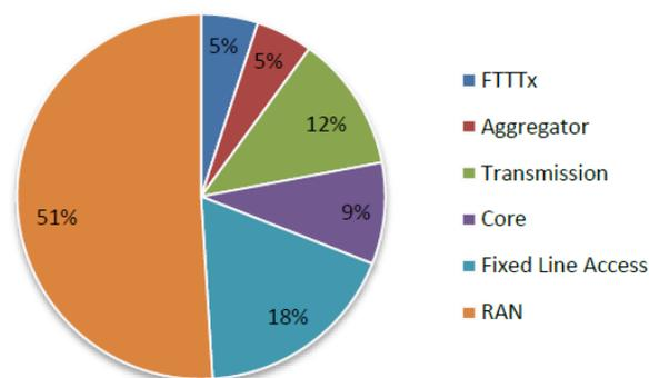
Figure 11. Distribution of power consumption across different network segments [78].
