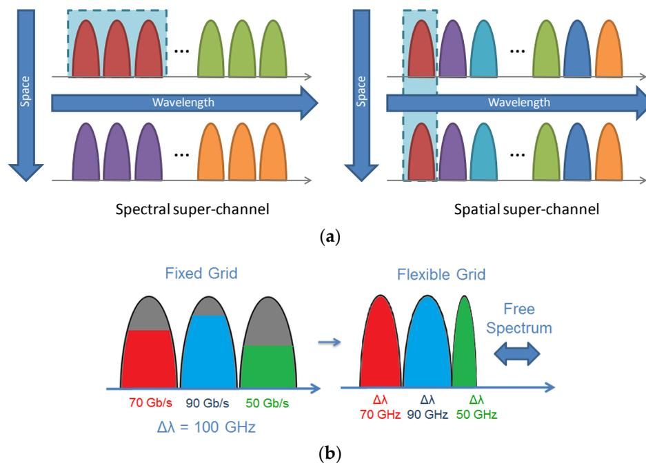
**Figure 6.** (a) Comparison of spatial and spectral super-channels. (b) Schematic representation of the advantages of flexible grids in terms of spectral efficiency.
