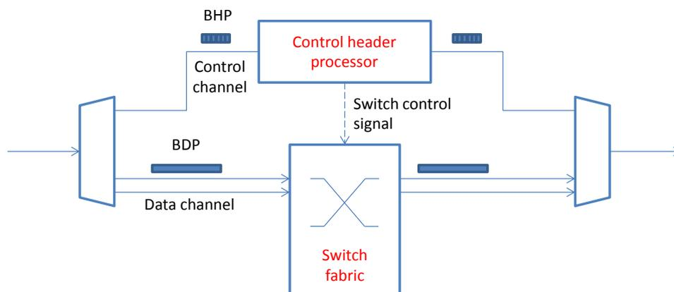
Figure 9. Schematic representation of an OBS router.
