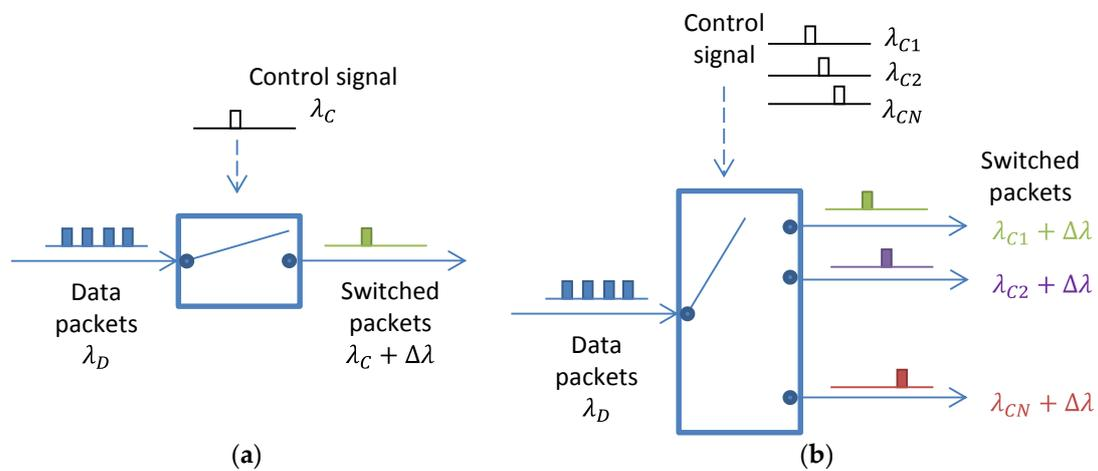
**Figure 10.** Schematic representation of the packet switching technique proposed by Hu et al. [75]: (a) one control wavelength; (b) different control wavelengths.
