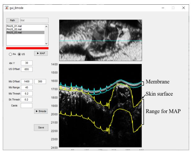
**Figure S4. Matlab based skin detection software with graphical user interfaces.** The blue and yellow lines denote the membrane and animal-body, respectively.
