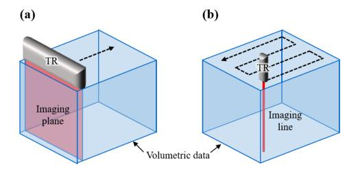
**Figure S1. Scanning methods for acquiring volumetric data.** (a) Volumetric data acquisition with the elevational scanning of a linear-array transducer. (b) Volumetric data acquisition with the raster scanning of a spherical single-element transducer. The black dashed lines represent the scanning paths. The red plane and line depict the imaging plane and imaging line with a single laser pulse. TR, transducer.
