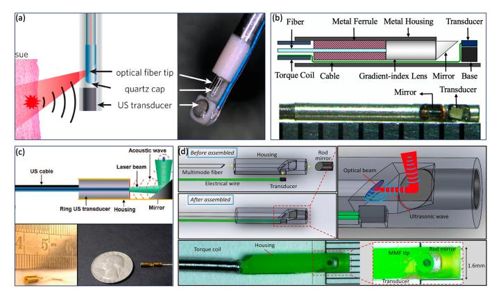
**Figure 4.** Intravascular imaging probe. (**a**) Sequential alignment and broad illumination. Adapted from [72]. (**b**) Sequential alignment and focusing illumination. Adapted from [22]. (**c**) Coaxial alignment and broad illumination. Adapted from [11]. (**d**) Coaxial alignment and broad illumination. Adapted from [70].
