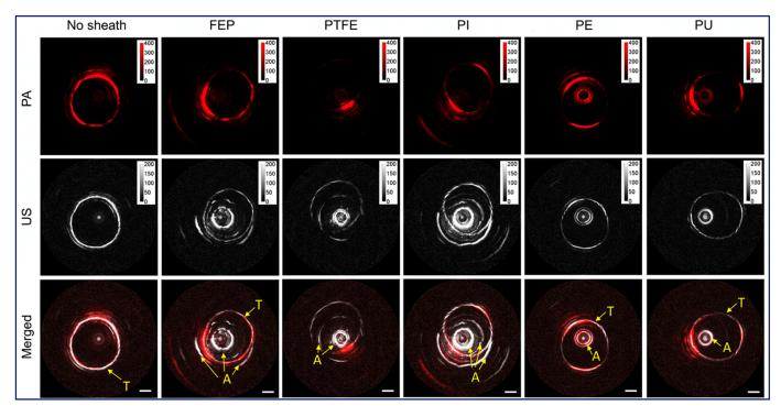
**Figure 5.** Sheath performance. Adapted from [89]. PE, polyethylene. FEP, fluorinated ethylene propylene. PTFE, polytetrafluoroethylene. PI, polyimide. PU, polyurethane. A, induced artifact from sheath. T, imaging target.
