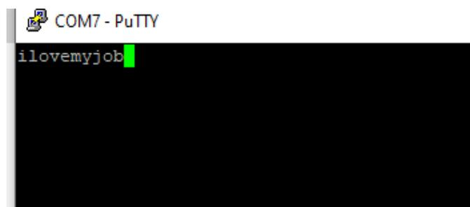
Figure 20. Text Characters successfully received at the UART reception port.
