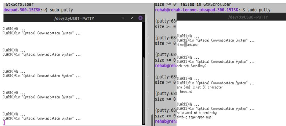
Figure 14. UART random text Communication between FPGA and PC.
