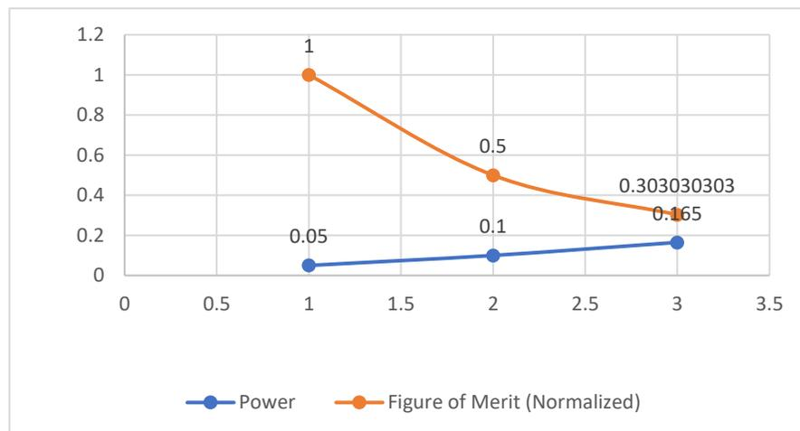
Figure 22. Figure of Merit (b/sW) change with power (W) at a fixed data rate.
