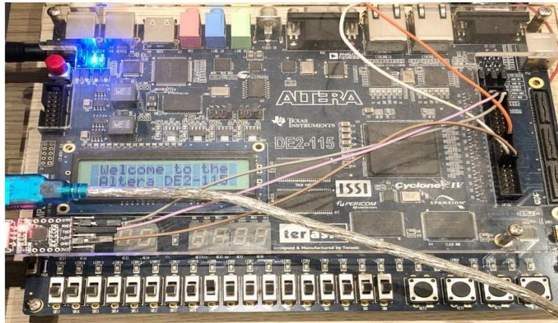
Figure 17. The ALTERA FPGA Kit of the proposed system.
