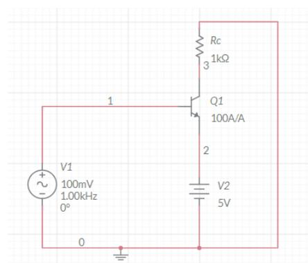
Figure 7. Initial testing driver circuit for TIP31C.
