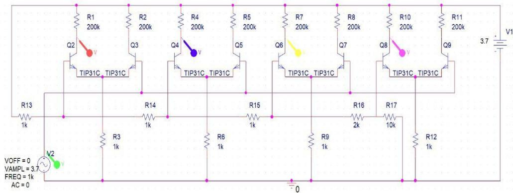
Figure 11. Demodulation Circuit.
