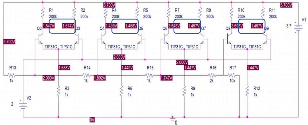
Figure 16. Receiver Circuit Simulation for 2 V input.
