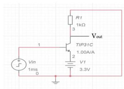
**Figure 5.** Laser Driver Circuit.
