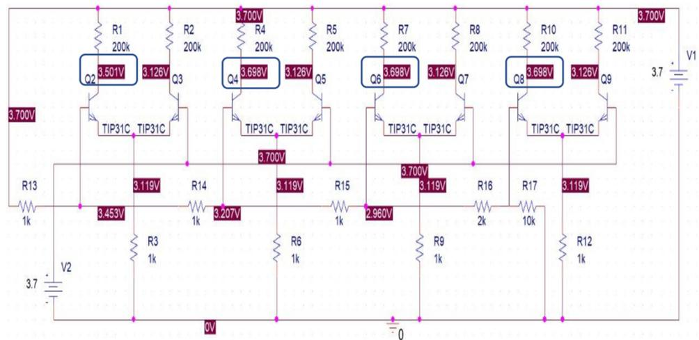
Figure 15. Receiver Circuit Simulation for 3.7 V input.
