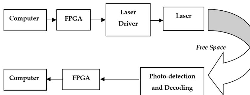
**Figure 2.** System Block Diagram.
