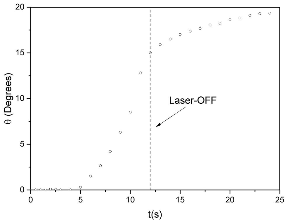
**Figure 6.** Angular displacement (Degs) as a function of time (s) for the black colored PVC tape when illuminated by the red laser at  $\lambda = 650$  nm. The dashed line indicates the point at which the red laser is switched off.
