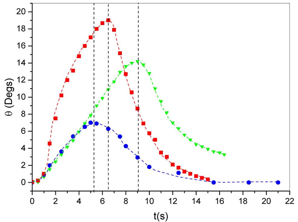
**Figure 5.** Angular displacement (Degs) as a function of time (s) for three different wavelengths,  $\lambda = 405$  (blue filled circles),  $532$  (green filled triangles), and  $650$  (red filled squares) nm. The dashed lines represents the points where the laser lights are switched off.
