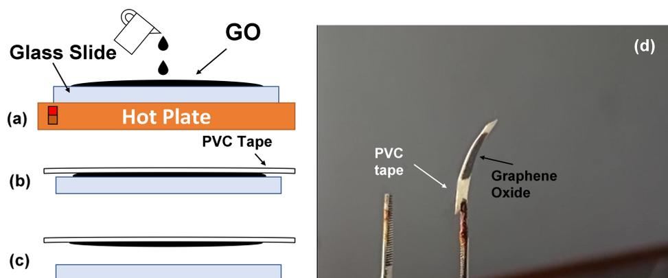
**Figure 2.** On the left side is a sketch of the preparation process. In (a), GO is deposited on a glass substrate placed on a hot plate at  $60\text{ }^{\circ}\text{C}$ . In (b), the PVC tape is placed in contact with the dried GO film, and in (c), the bilayered structure is detached from the substrate. On the right side (d) is the final result.
