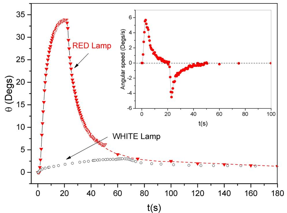
**Figure 4.** Angular displacement of the film as function of time when incoherent illumination is used. Different sources give completely different results. In the inset is the angular velocity corresponding to the NIR red lamp.
