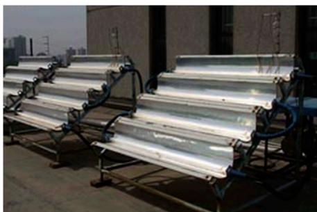
**Figure 30.** CPC based direct solar photoreactor for hydrogen production. Reproduced with permission from [120]. Copyright Elsevier, 2010.
