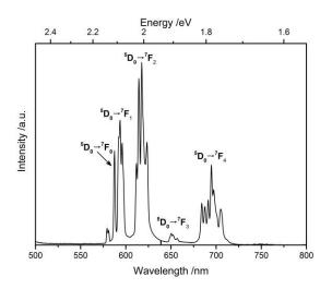
**Figure 5.** Emission spectrum of a  $\beta$ -Y<sub>2</sub>B<sub>4</sub>O<sub>9</sub>:Eu<sup>3+</sup> (8%) single-crystal obtained upon excitation at 448 nm.
