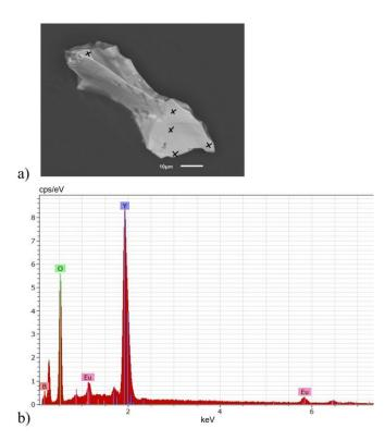
**Figure 4.** (a) Crystal used for the EDX measurement (crosses indicate the measured positions); (b) EDX spectrum of  $\beta$ -Y<sub>2</sub>B<sub>4</sub>O<sub>9</sub>:Eu<sup>3+</sup> (8%). The unindexed peak at ~0.3 keV originates from carbon used for the sputtering process.
