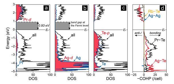
**Figure 2.** Densities-of-states (DOS) and crystal orbital Hamilton population (COHP) curves of RbPr<sub>2</sub>Ag<sub>3</sub>Te<sub>5</sub>: the Fermi level,  $E_F$ , is given by the black horizontal line, while the atom-projected DOS (blue) of praseodymium, silver, and tellurium are shown in (**a**)–(**c**), respectively. Additionally, the orbital-projected DOS (red) which provide the largest contributions to the states near  $E_F$  for a given sort of atom have been included.
