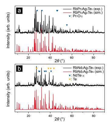
**Figure 3.** Measured and simulated powder X-ray diffraction patterns of (**a**) RbPr<sub>2</sub>Ag<sub>3</sub>Te<sub>5</sub> and (**b**) RbNd<sub>2</sub>Ag<sub>3</sub>Te<sub>5</sub>: reflections corresponding to the by-products, i.e., Pr<sub>7</sub>O<sub>12</sub> [41], NdTe<sub>1.8</sub> [42,43], and tellurium [44], have been denoted by the different triangles.
