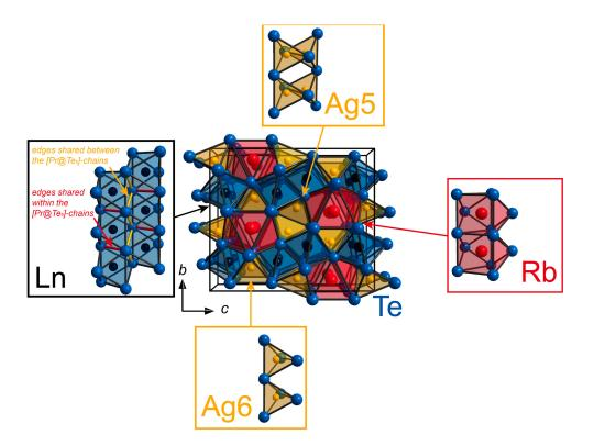
**Figure 1.** View on the unit cell of  $RbLn_2Ag_3Te_5$  (Ln = Pr, Nd) along *a*: the crystal structures of the tellurides are composed of tunnels which are assembled by the tellurium atoms and enclose the rubidium, lanthanide, and silver atoms, respectively. The diverse types of tellurium (blue) polyhedra surrounding the rubidium (red), lanthanide (black), and silver atoms (orange) are shown in the insets.
