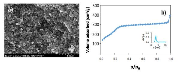
**Figure 1.** (a) SEM image of calcined mesoporous silica nanoparticles (MSNs) showing the narrow particle size distribution, and (b) the nitrogen sorption isotherm measured at 77 K for the same particles. The inset in Figure 1b shows the pore size distribution plot.
