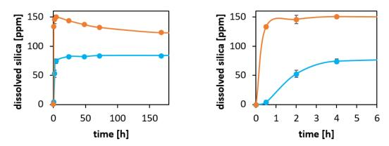
**Figure 4.** Left: Silicon concentrations measured by ICP-OES as a function of incubation time in PBS (pH = 7.2) at 37 °C. Orange dots: 5 mg particles/mL, blue dots: 0.1 mg particles/mL. Right: Zoom highlighting the early stages of dissolution. The lines are guides for the eye.
