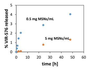
**Figure 3.** Release of VIR-576 into PBS buffer from MSNs having an initial VIR-576 loading of 11.5 wt % as a function of particle concentration. T = 25 °C. Error =  $\pm 0.2$ %-units.
