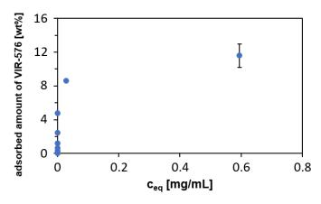
**Figure 2.** Adsorption isotherm of VIR-576 adsorbed onto MSNs from PBS (pH = 7.2). Particle concentration: 5 mg/mL, temperature =  $25 \degree C$ , and incubation time = 1 h.
