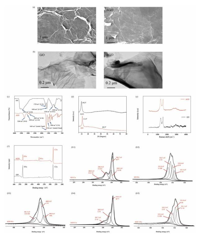
**Figure 1.** Characterization of amidated graphene oxide (AGO). (a) SEM, (b) TEM, (c) FTIR spectra, (d) XRD pattern, (e) Raman spectra, (f) XPS survey spectra, (f-1) C1s spectra of GO, (f-2) O1s spectra of GO, (f-3) N1s spectra of AGO, (f-4) C1s spectra of AGO, and (f-5) O1s spectra of AGO.
