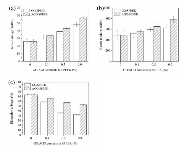
Figure 3. Mechanical properties of AGO/SPEEK films. (a) Tensile strength, (b) elastic modulus, (c) elongation at break.
