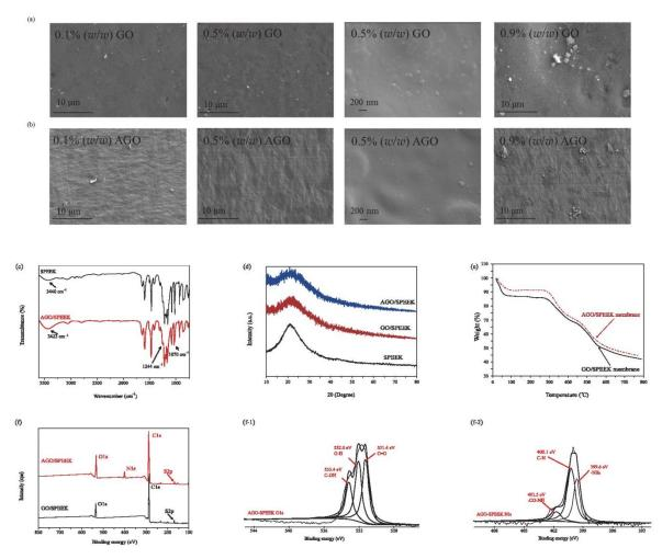
**Figure 2.** Characterization of films. (a) SEM of GO/SPEEK films, (b) SEM of AGO/SPEEK films, (c) FTIR spectra, (d) XRD pattern, (e) TGA curves, (f) XPS survey spectra, (f-1) O1s spectra and (f-2) N1s spectra of 0.5% (*w/w*) AGO/SPEEK films.
