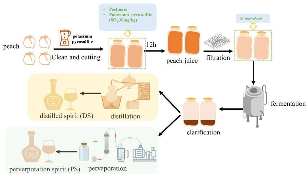
**Figure 1.** A process flow of DS and PS production.
