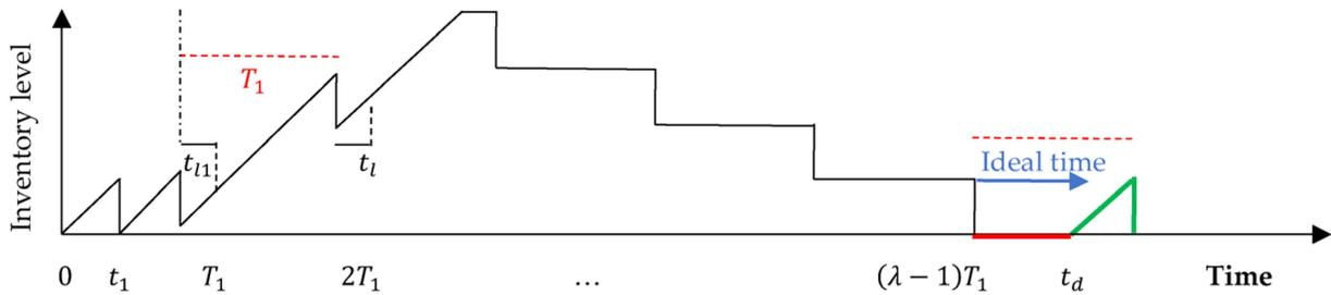
Figure 3. Inventory status of the joint model for the vendor in the first cycle.
