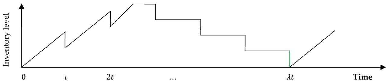
**Figure 1.** Inventory status of the classical joint model for the vendor in any given cycle.
