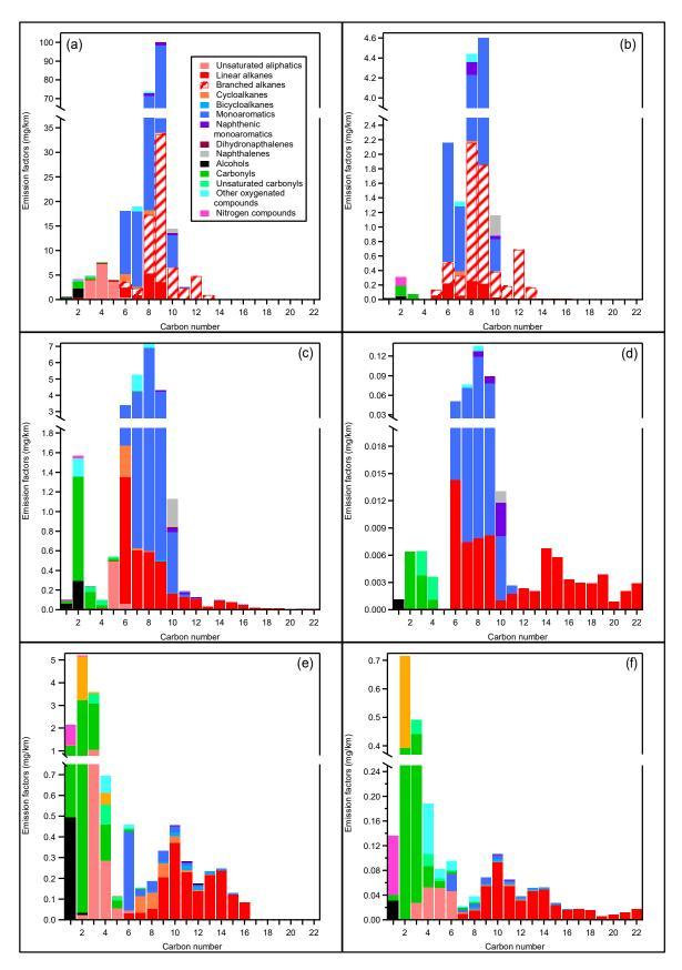
**Figure 4.** NMVOC EFs in mg/km as a function of carbon numbers for a typical (a) GDI CU cycle, (b) GDI MW cycle, (c) PFI CU cycle, (d) PFI MW cycle, (e) diesel CU cycle, and (f) diesel MW cycle. The different colors correspond to the main chemical classes measured by PTR-ToF-MS and GC-MS.
