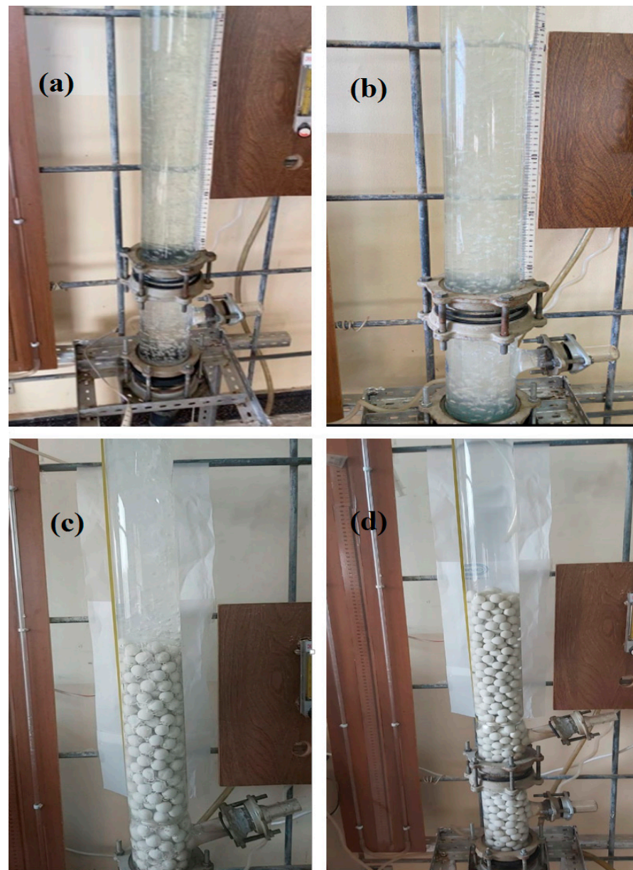
Figure 3. Photos of the reaction apparatus of the BCR applying the four experimental methods: (a) O_3 gas alone, (b) O_3 /ZnO nanocatalyst, (c) O_3 / Al_2O_3 , and (d) O_3 / Al_2O_3 /ZnO nanocatalyst.
