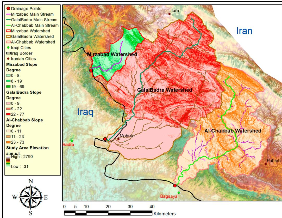
**Figure 3.** Characteristics of terrain elevation, main stream, and terrain slope of Mirzabad, Galal Badra, and al-Chabbab watersheds.
