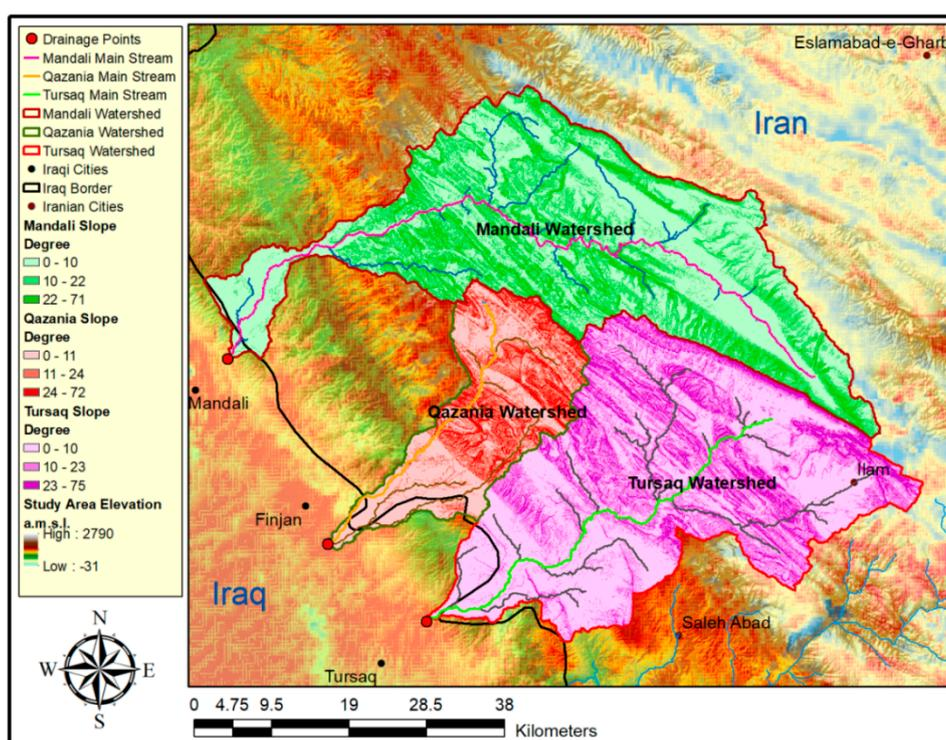
**Figure 2.** Characteristics of terrain elevation, main stream, and terrain slope of Mandali, Qazania, and Tursaq watersheds.
