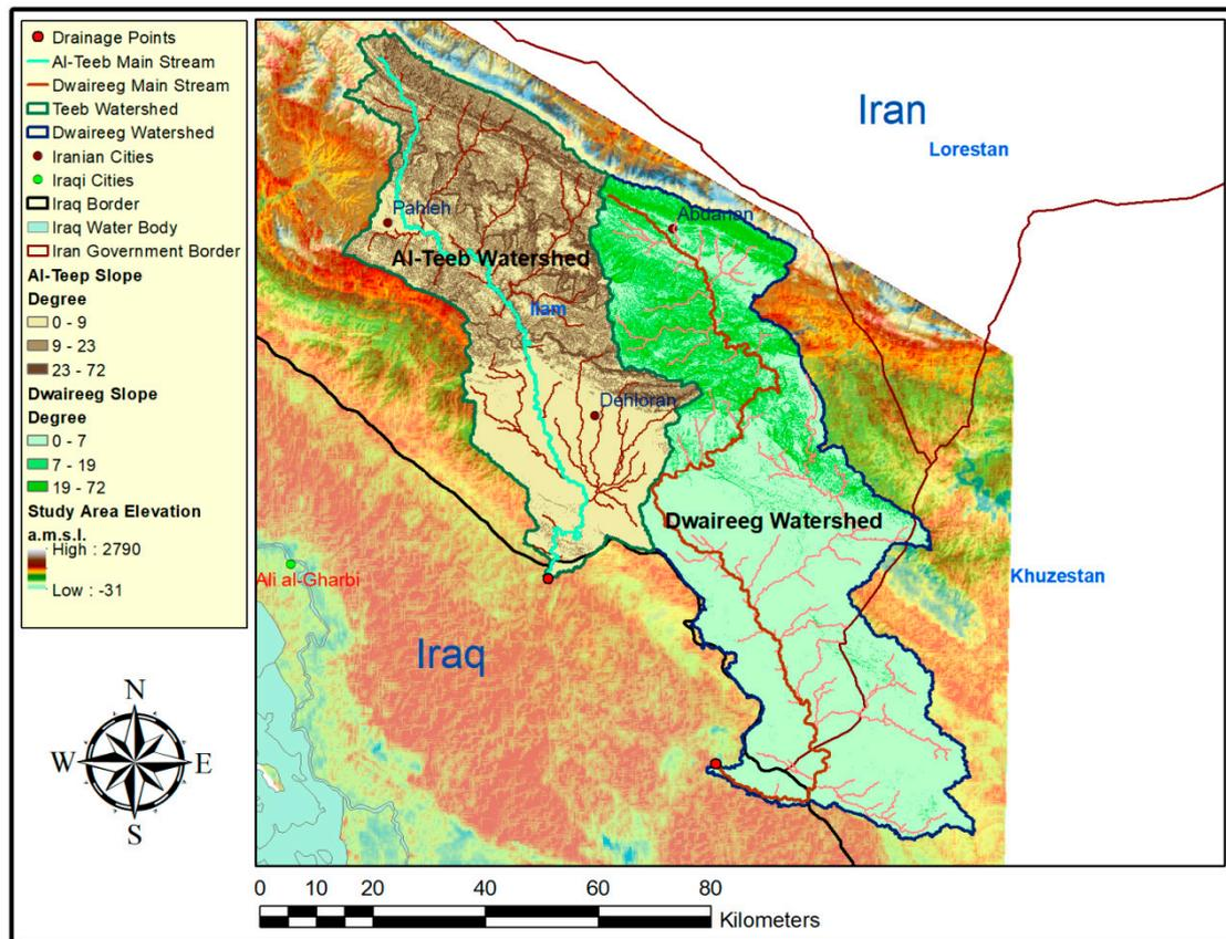
**Figure 4.** Characteristics of terrain elevation, main stream, and terrain slope of al-Teeb and Dwaireeg watersheds.
