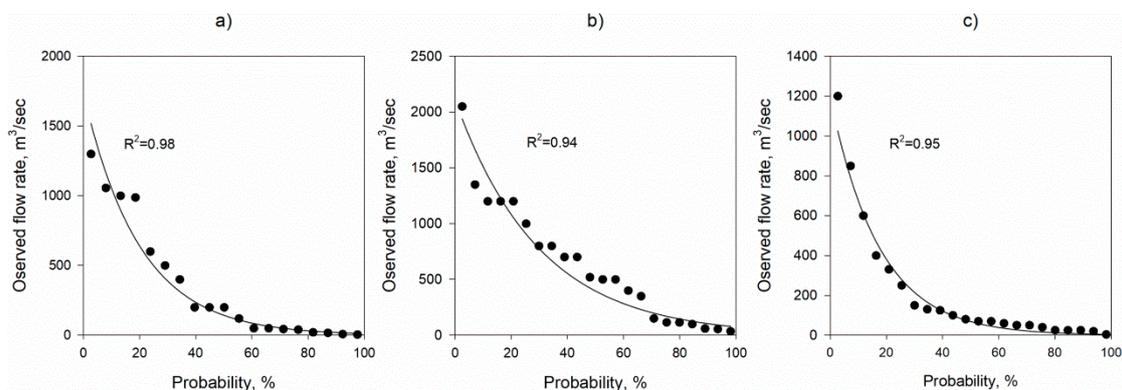
**Figure 7.** Statically analyzed using normal probability plots of observed flow rates for the three streams: (a) Tursaq, (b) Galal Badra, and (c) al-Chabbab.
