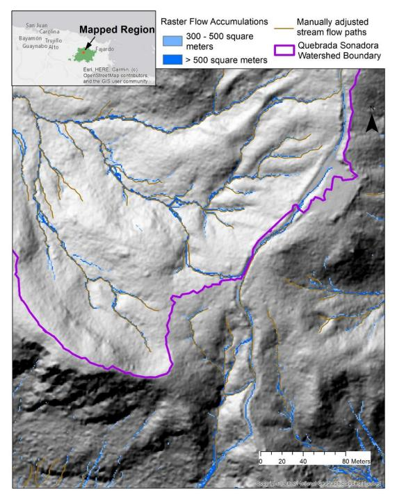
**Figure 6.** Here we show the raster based flow accumulation down to 300 m<sup>2</sup>, with the manually adjusted stream flow path features in brown. This level of detail is not practical at the landscape scale due to the amount of effort it would require. However, was done here for an intensively studied Quebrada Sonadora watershed.
