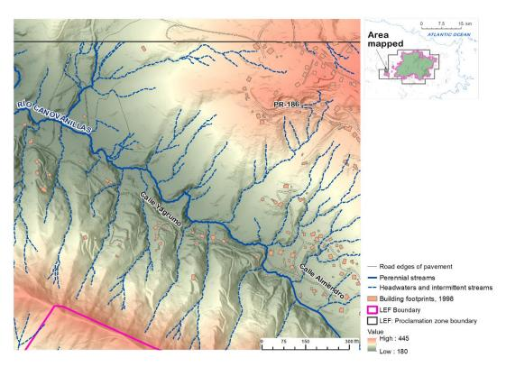
**Figure 7.** Example of headwaters, intermittent flow paths, and perennial channels derived from a threshold  $\geq$ 5000 accumulated cells (0.5 ha).
