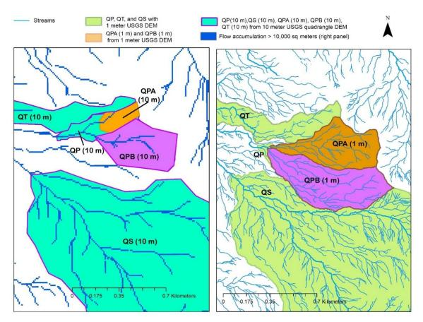
**Figure 5.** Map of streams in the El Verde Research area. Left panel contains stream networks derived from 10 square meter DEM from USGS quadrangle maps, right panel includes streams derived from 1 square meter USGS DEM. Watersheds derived from 10 m DEM are labeled (10 m). The watersheds outlined are QT: Quebrada Toronja; QP: Quebrada Prieta; QPA: Quebrada Prieta A; QPB: Quebrada Prieta B; QS: Quebrada Sonadora.
