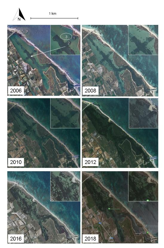
**Figure 10.** Sequence of aerial photographs (time span from 2006 to 2018), showing evolution of the sinkhole phenomena.
