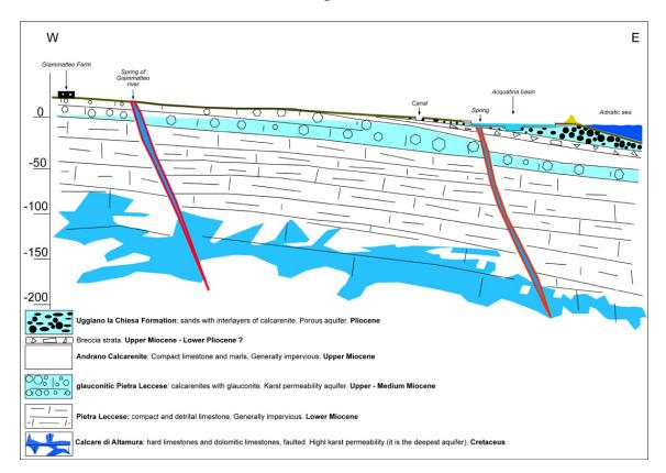
**Figure 7.** Schematic hydrogeological section of the studied area (not in scale). For the trace of the section see Figure 6. Red sub-vertical lines are faults, whilst the blue colors in the section indicate the presence of groundwater.
