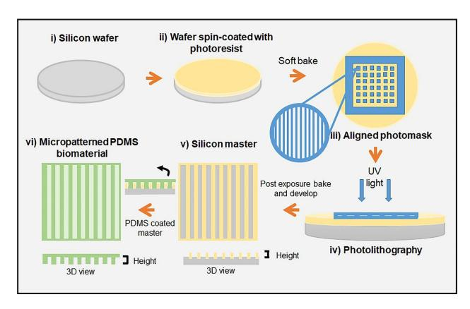
**Figure S1.** Soft lithography protocol for fabrication of micropatterned PDMS biomaterial. The photoresist viscosity and parameters for spin-coating speed, soft bake temperature, photolithography exposure, and post exposure temperature were dependent on the desired three-dimensional pattern height.
