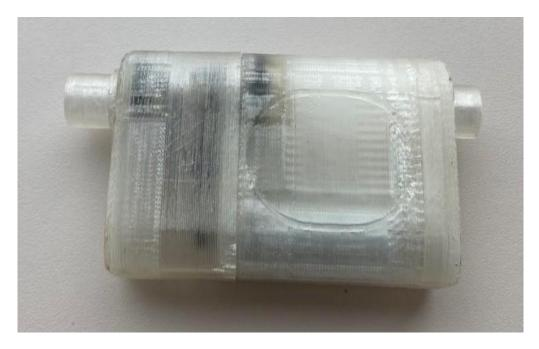
Figure 7. Prototype of the device made using fused deposition modeling technique.
