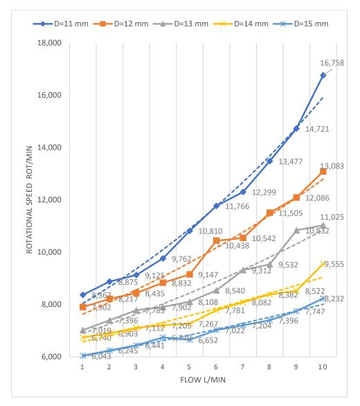
**Figure 3.** Graphical representation of the values of rotational speeds required for different pump diameters to provide different flow rates calculated by mathematical modeling and approximated on the Cordier diagram. D, diameter.
