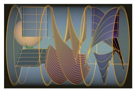
**Figure 4.** Resulting 3D geometries of the pump. From left to right: inducer (black), impeller (red), diffuser (purple).
