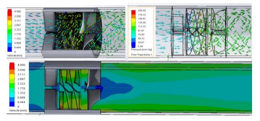
**Figure 5.** CFD analysis shows flow trajectories (**top**) with velocities (**top left**), pressures (**top right**) and trans-axil plane velocities (**bottom**).
