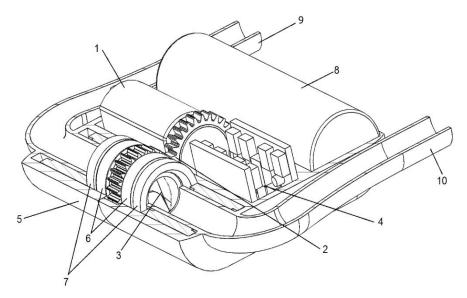
**Figure 2.** The implantable system of the device—section through the housing. Legend: 1: motor, 2: mechanical transmission, 3: pump rotor, 4: electronic circuit, 5: housing, 6: bearings, 7: sealing elements, 8: battery, 9: outflow cannula, 10: inflow cannula.
