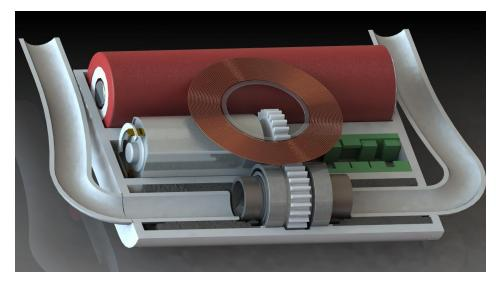
**Figure 6.** Longitudinal section through the implant including battery, motor, transmission, pump, antenna, suction, and discharge.
