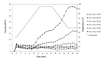
**Figure 2.** Rapid Visco-Analyser pasting curve of starting soybean–navy bean blends with different ratios.
