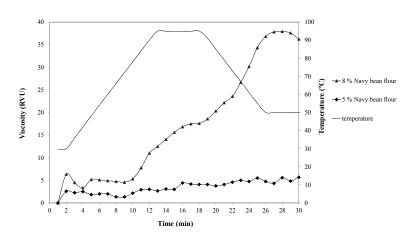
Figure 3. Rapid Visco-Analyser pasting curve of navy bean with 5% and 8% solids.
