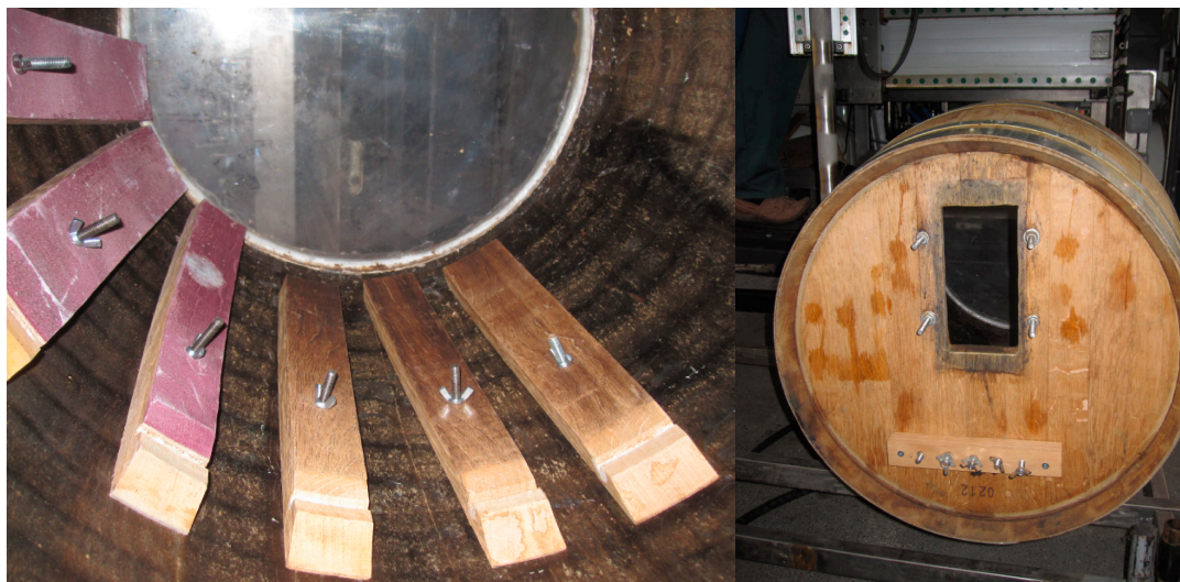
Figure 2. Experimental barrel for HPU treatment.
