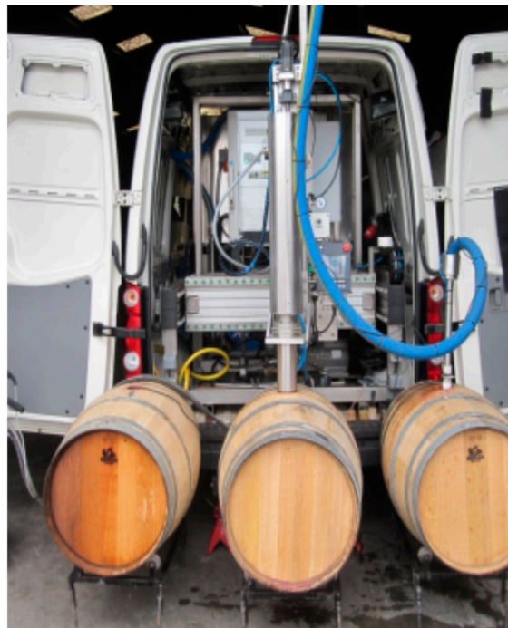
Figure 1. High power ultrasound (HPU) apparatus.
