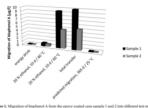
**Figure 1.** Migration of bisphenol A from the epoxy-coated cans sample 1 and 2 into different test media and calculated migration at the end of shelf life.
