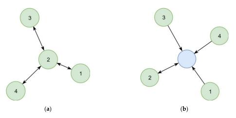
**Figure 6.** Two representations of four synonym identifiers (1–4) in a graph. (**a**) Links between identifiers indicate known synonym relationships. Synonyms of an identifier are all directly or indirectly connected other identifiers. (**b**) Identifiers point to the identified chemical (blue circle). All identifiers pointing to the same chemical are synonyms. The chemical has a preferred identifier (double arrow).
