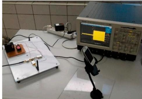
**Figure 2.** Data acquisition system with radio frequency (RF) front end.
