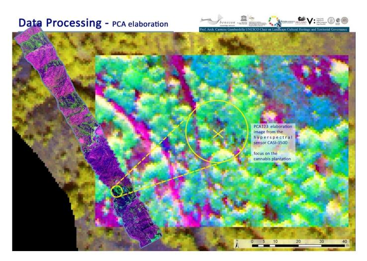
**Figure 4.** False color representation PCA (principal components analysis), sampled according to the statistical processing of the acquired electromagnetic bands that maximizes the variance of the spectral data and filters the electromagnetic noise.
