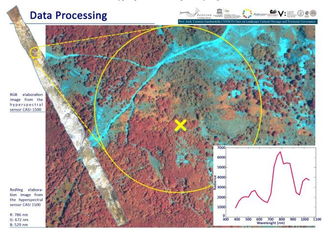
**Figure 3.** From the ortho-corrected images the protocol considers two type of elaboration: the RGB "true color" elaboration and the "Red-Veg" elaboration, wherein the cannabis plant is enhanced. Moreover, the spectral signature is extracted.
