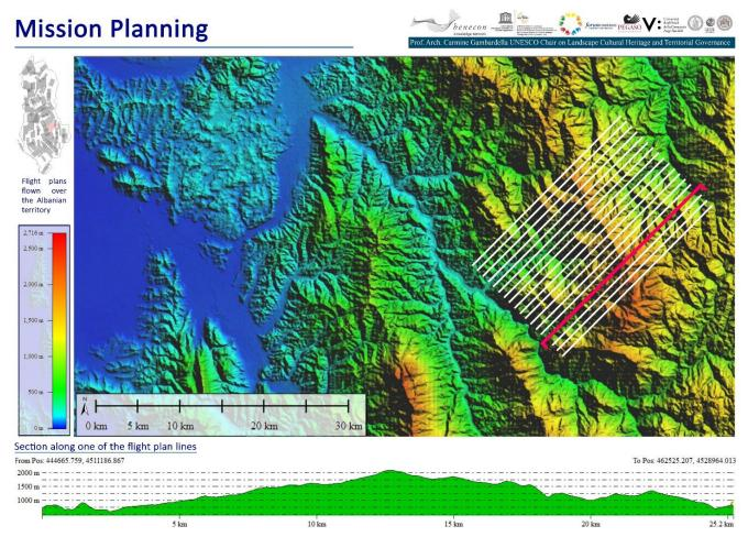
**Figure 1.** Mission planning: focus on a flight plan designed over the southeast of the Albanian territory. Each flight plan is specifically designed taking into consideration the orography of the territory to fly over. Software used: Global Mapper.
