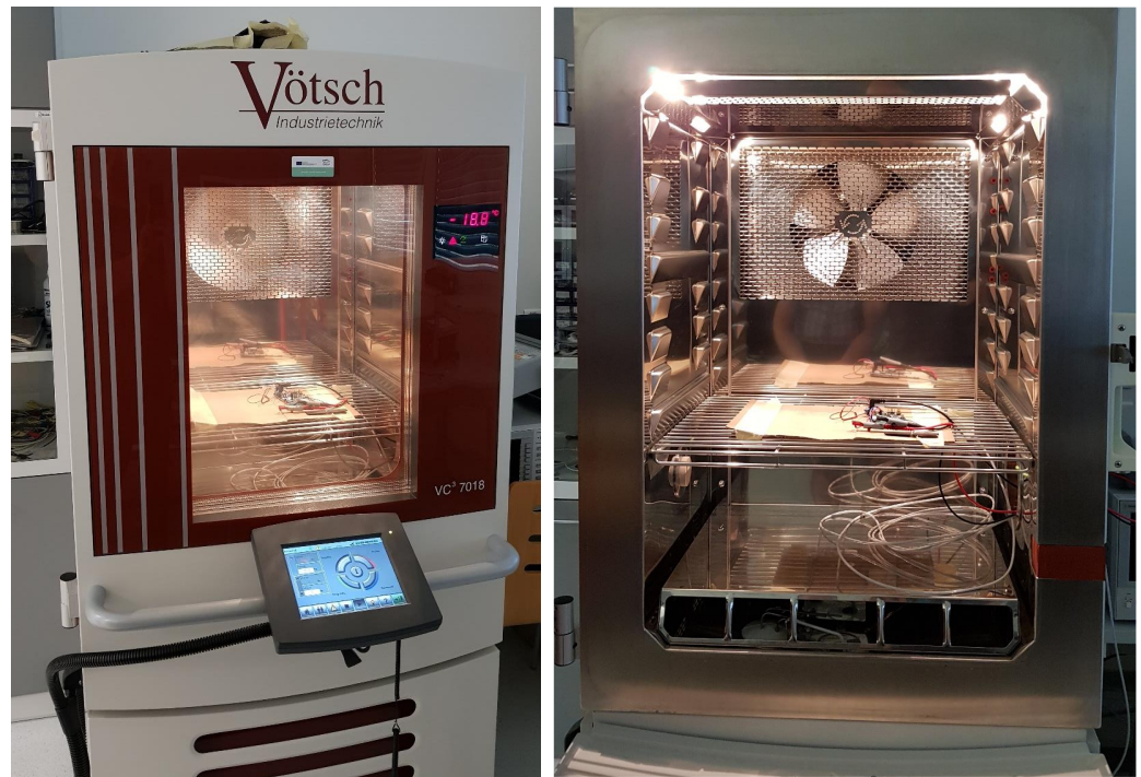
Figure 4. Durability measurements of devices in different climatic conditions in the temperature chamber Vötsch VC3 7018.
