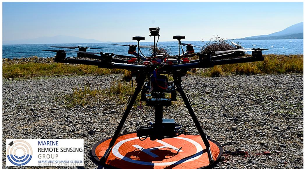
**Figure 9.** DJI S1000 with Bayspec OCI-F on a custom-made gimbal.
