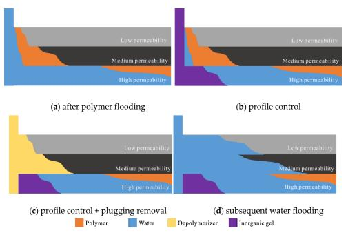
**Figure 12.** Action mechanism of "profile control + plugging removal" (**a**) after polymer flooding, (**b**) profile control, (**c**) profile control + plug removal and (**d**) subsequent water flooding.
