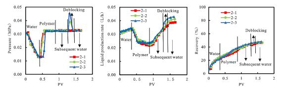
Figure 6. Relationships between injection pressure, liquid production rate, and recovery, and PV.
