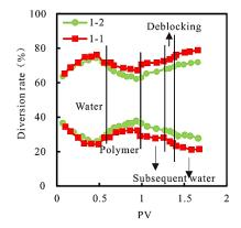
Figure 5. Relationship between diversion rate and PV at production end.
