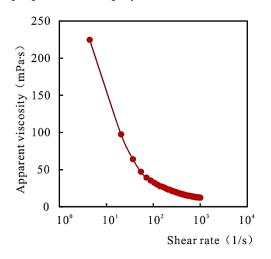
Figure 1. Relationship between polymer shear time and apparent viscosity.
