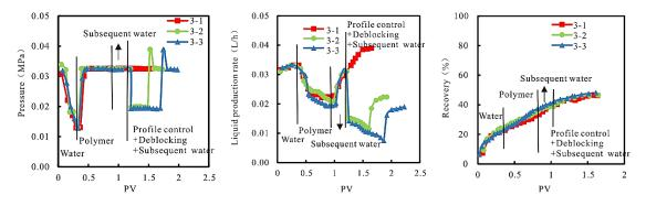
Figure 7. Relationships between injection pressure, production rate, and recovery, and PV.
