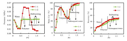
Figure 4. Relationship between injection pressure, water cut, and recovery and PV.
