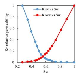
Figure 9. Oil-water relative permeability curve.
