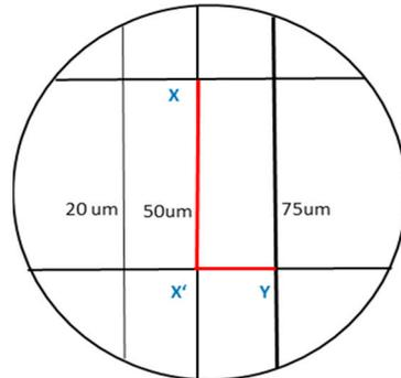
**Figure 6.** Schematic drawing of the stainless-steel analog indicating the lines measured between reference points X-X' (Vertical dimension) and X'-Y (horizontal dimension).
