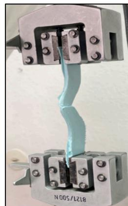
**Figure 7.** Tear strength specimen clamped in a Zwick testing machine.
