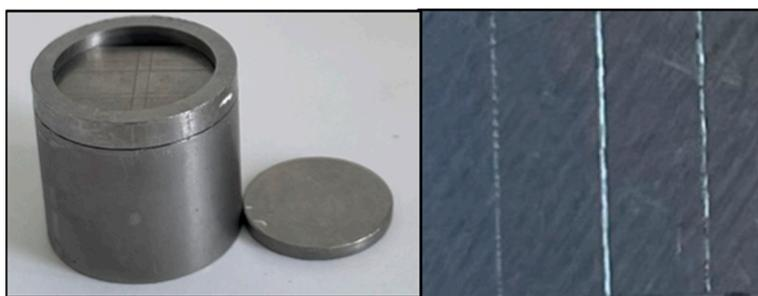
**Figure 5.** Detail reproduction metal mold with 20, 50, and  $75\text{ }\mu\text{m}$  depth engraved lines.
