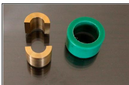
**Figure 8.** Copper split mold and a plastic fixation ring for elastic recovery testing.
