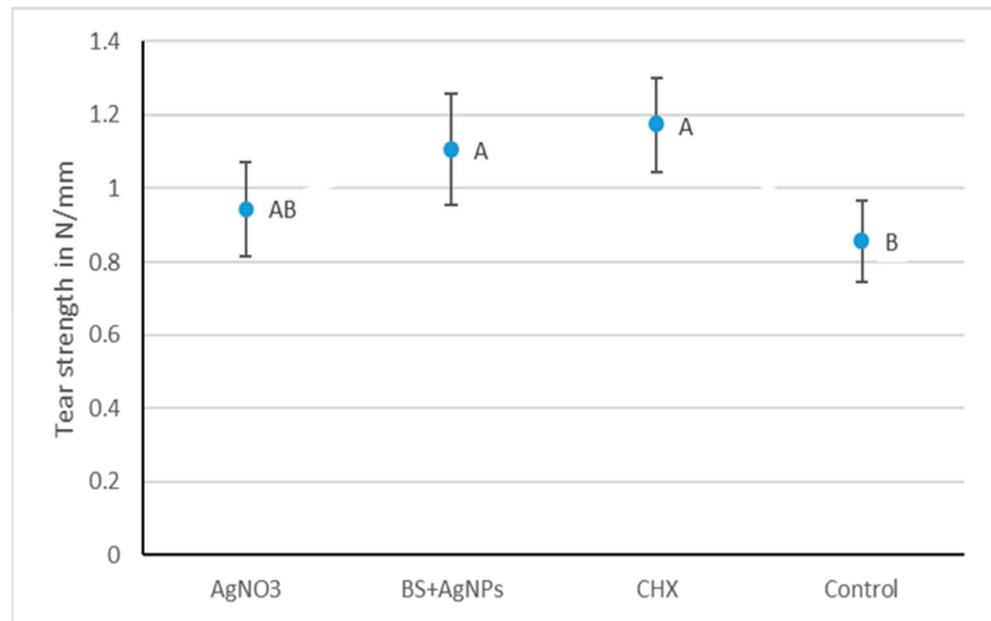
**Figure 3.** Interval plot representing the mean tear strength (N/mm) values and 95% confidence interval of all tested groups. Groups that do not share a letter are significantly different.
