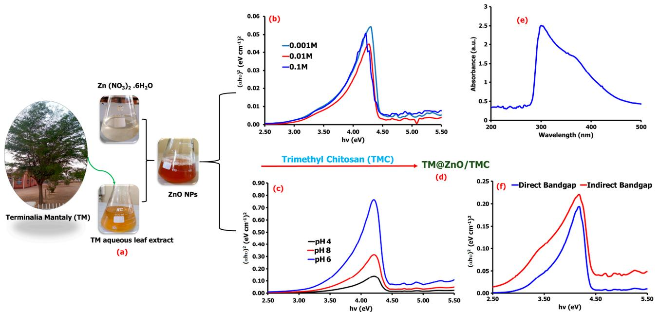
**Figure 1.** Schematic representation of the synthesis of ZnO NPs from TM leaf extract (a), the direct and indirect bandgap energies of the synthesized TM@ZnO NPs at varying concentrations of the precursor salts (b) and pH (c). The produced TM@ZnO/TMC NC hydrogel product (d), its UV-vis spectrum (e), and the corresponding bandgap spectra (f).
