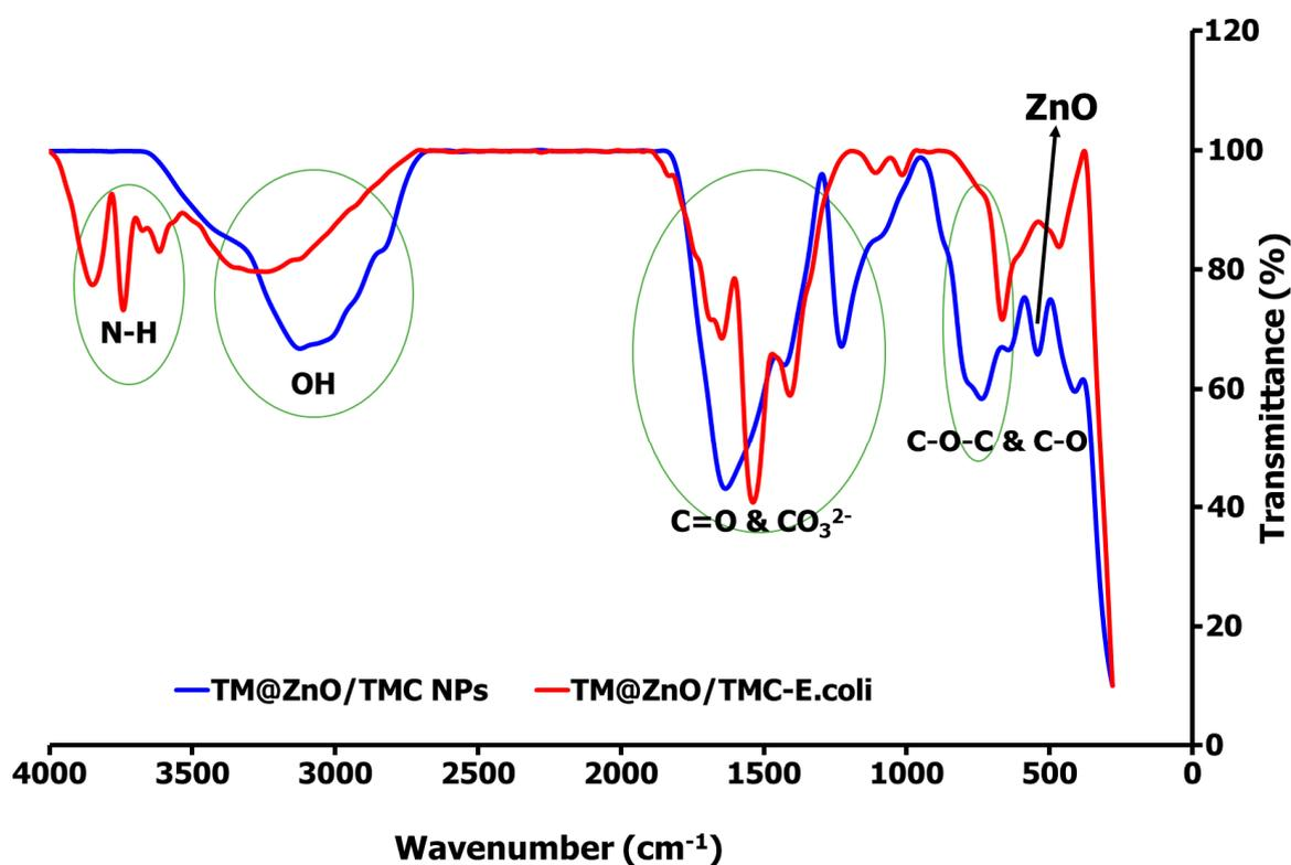
**Figure 6.** FTIR spectral comparison of TM@ZnO/TMC NC hydrogel before and after interaction with *E. coli*, demonstrating the adsorption mechanism.
