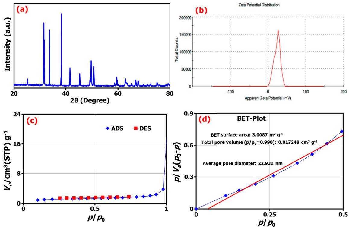
**Figure 3.** (a) The XRD pattern, (b) the zeta potential from DLS analysis, (c) the adsorption/desorption isotherms, and (d) BET analysis of TM@ZnO/TMC NC hydrogel.
