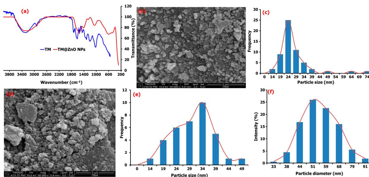
**Figure 2.** (a) FTIR analysis of pure TM leaf extract compared to TM@ZnO NC hydrogel, (b) the FESEM image and (c) particle size distribution of TM@ZnO NPs. (d) FESEM macrograph, Mag  $\times$  50,000 (e) particle size distribution, and (f) DLS particle diameter of TM@ZnO/TMC NC hydrogel.
