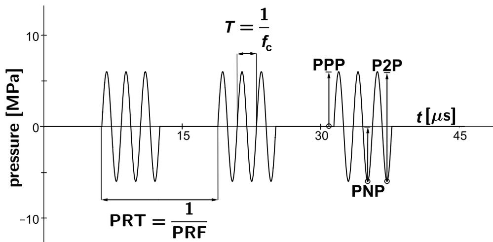
**Figure 2.** Representation of an ultrasound pulse sequence with dominant period  $T$ , centre frequency  $f_c$ , peak-positive pressure (PPP), peak-negative pressure (PNP), peak-to-peak pressure (P2P), pulse-repetition period (PRT), and pulse-repetition frequency (PRF).
